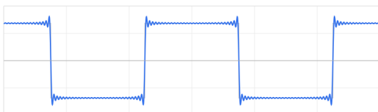
Ringings when a square wave is approximated using a finite number of frequency components
