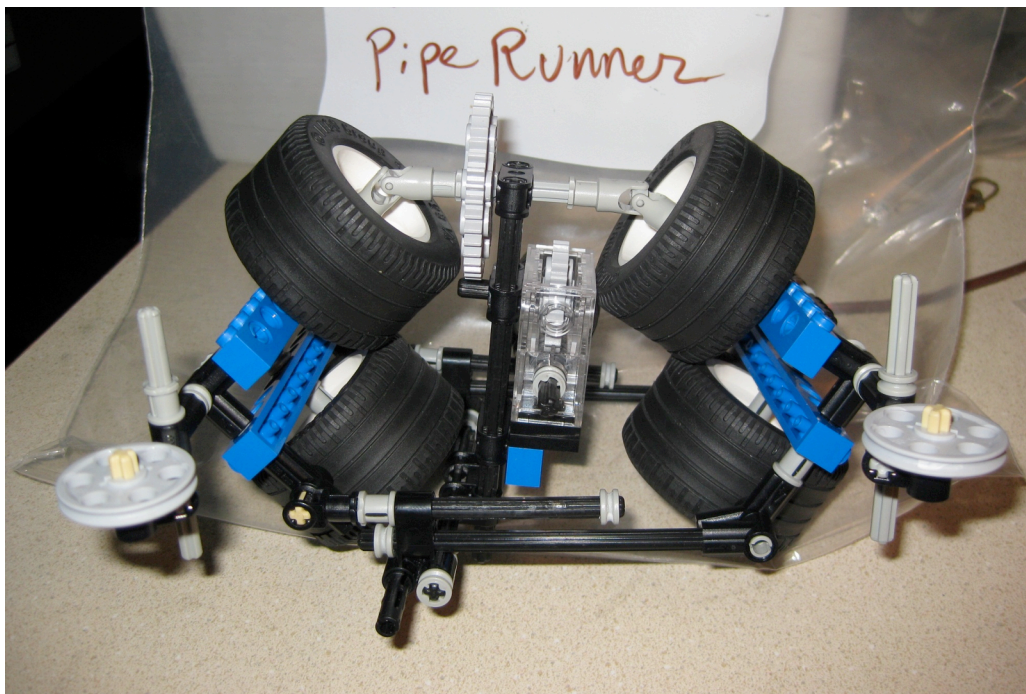
Figure 7: The experimental unit, sporting an unbiased orientation drive system
