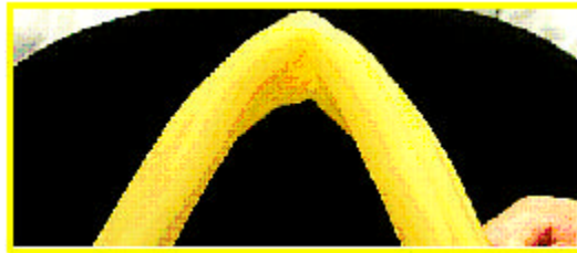
Figure 23: Representation of kinking problem when device is attached to calf
