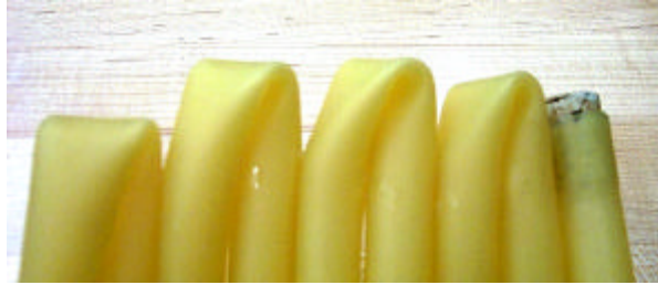
Figure 22: Kinking problem when winding tubing around
