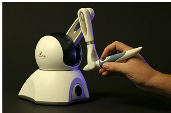
Fig. 42.5 The Phantom Omni device from SensAble Technologies, now marketed as the Geomagic Touch. This relatively low-cost device senses motion in six degrees of freedom from the stylus and can apply forces in the x , y , and z directions to the stylus tip (courtesy SensAble Technologies, Inc., Woburn)
