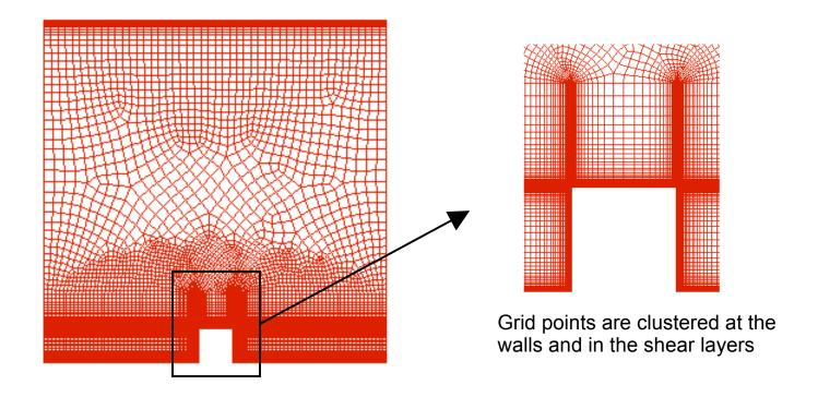
Unstructured gridding allows to separate the bottom and top BLs having different resolutions in the streamwise direction
