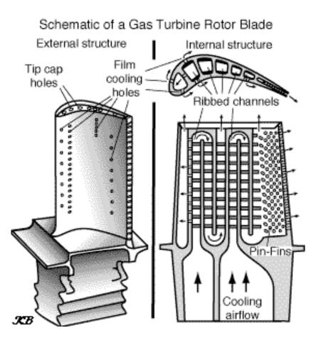
Turbulence is enhanced is internal turbine cooling passages to improve heat transfer
