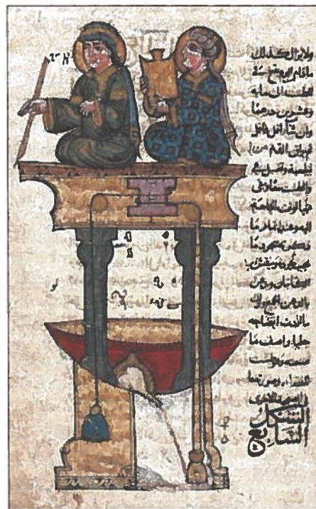
The Basin of the Scribes (a device to specify the exact amount of blood taken from a patient), from al-Jazari’s The Book of Knowledge of Ingenious Mechanical Devices (1315)
