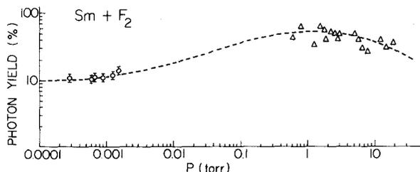
FIG. 9. Absolute photon yields as a function of pressure for the  $\text{Sm} + \text{F}_2$  reaction: (○) this work; and (△) Ref. 3. The dashed line is drawn to connect smoothly the low and high pressure data; no model is implied.
