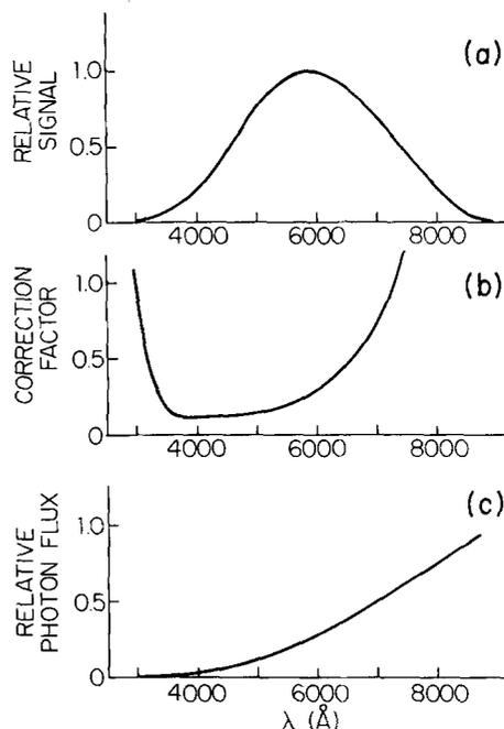
FIG. 3. (a) The spectrum of the standard lamp output,<sup>8</sup> which is multiplied by the correction factor (b) to obtain (c) the relative photon flux of the standard lamp. In practice, (a) and (c) are known, while (b) is derived.
