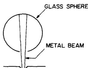
FIG. 5. Metal flux determination using a thin, hollow, glass sphere. In order to obtain a weighable sample the orifice of the entrance port to the scattering chamber is enlarged. While the number of metal atoms/sec that are collected increases, the flux (number of metal atoms/cm<sup>2</sup> sec) is not altered by the small change made.
