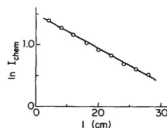
FIG. 7. Plot of the logarithm of the chemiluminescent intensity vs path length for the reaction  $\text{Sm} + \text{N}_2\text{O}$ . The data presented give a determination of  $\sigma_{\text{tot}} = 91 \text{ \AA}^2$ , which was included in the average reported in Table III.
