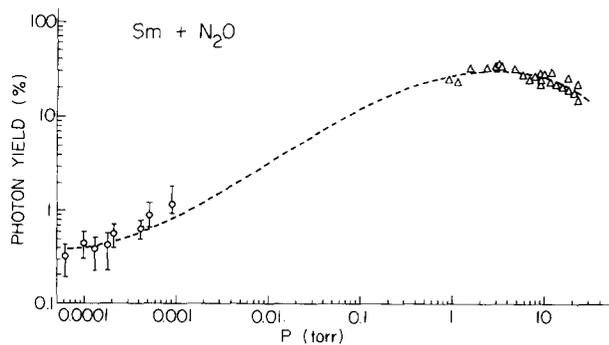
FIG. 8. Absolute photon yields as a function of pressure for the  $\text{Sm} + \text{N}_2\text{O}$  reaction: (○) this work; and (△) Ref. 3. The dashed line is drawn to connect smoothly the low and high pressure data; no model is implied.
