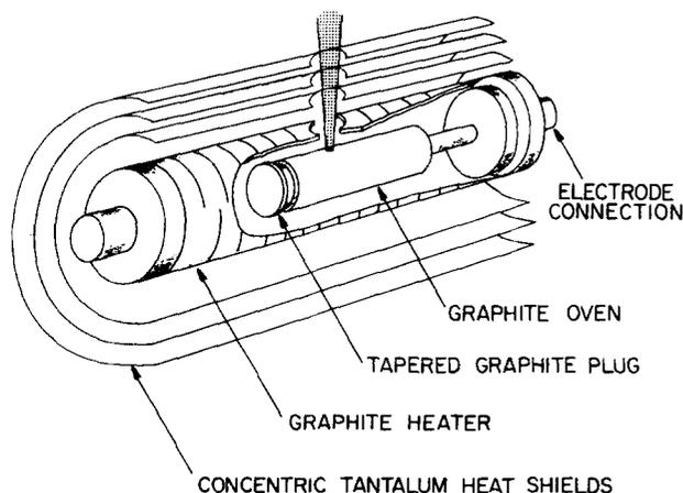
FIG. 2. Metal atom source, designed by R. C. Oldenborg.<sup>7</sup> A few hundred amperes are passed through a graphite cylinder, held between two water-cooled copper bussbars. The graphite heater has slots cut on its body to increase the resistance. Inside the heater and supported from one end is a graphite crucible containing the metal sample.
