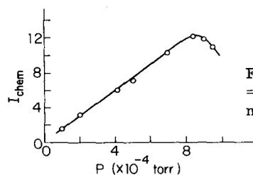
FIG. 6. Determination of  $\sigma_{\text{tot}} = 82 \text{ \AA}^2$  from the pressure maximum for  $\text{Sm} + \text{N}_2\text{O}$ .
