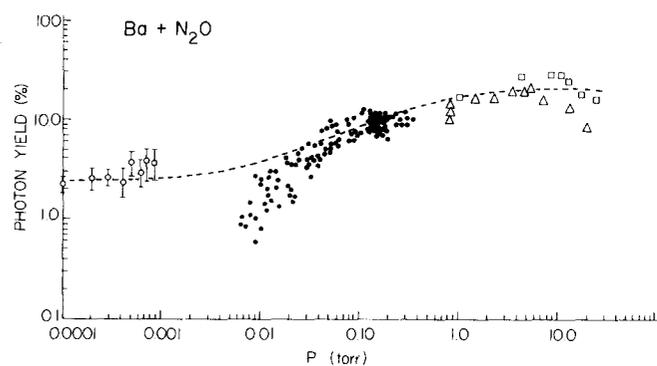
FIG. 10. Absolute photon yields as a function of pressure for the  $\text{Ba} + \text{N}_2\text{O}$  reaction: (○) this work; (●) Ref. 11; (△) Ref. 3; and (□) Ref. 6. The dashed line is drawn to connect smoothly the low and high pressure data; no model is implied.
