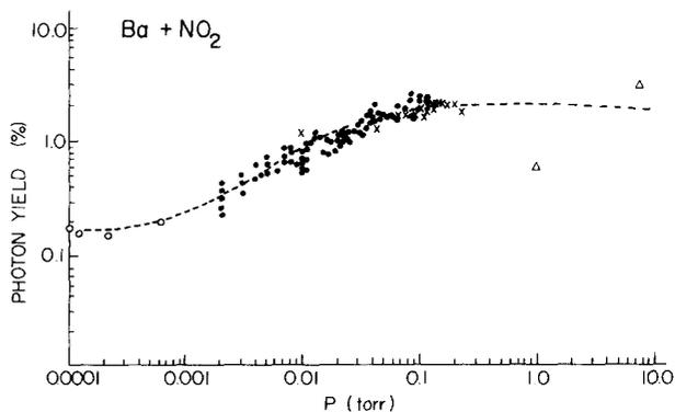
FIG. 11. Absolute photon yields as a function of pressure for the  $\text{Ba} + \text{NO}_2$  reaction: (○) this work; (●) and (×) Ref. 11; and (△) Ref. 6. The dashed line is drawn to connect smoothly the low and high pressure data; no model is implied.
