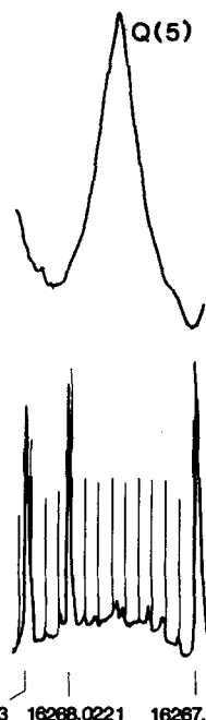
FIG. 2. High-resolution laser optogalvanic trace of the Q(5) line of the HCO \bar{A}(0, 9^0, 0) \rightarrow \bar{X}(0, 0^1, 0) band. The lower trace shows the simultaneous recording of the fluorescence excitation of I_2 , as well as fringes from a 1.97 GHz etalon used for calibrating the wavelength. The wave numbers 16267.8013 and 16268.0221 \text{cm}^{-1} attached to the I_2 calibration lines on the left side of Fig. 2 should be interchanged.
