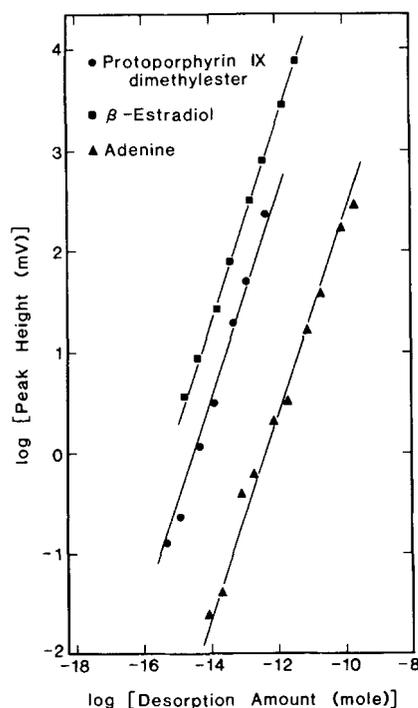
Figure 2. Parent ion signal for protoporphyrin IX dimethyl ester,  $\beta$ -estradiol, and adenine vs. amount desorbed per laser pulse.
