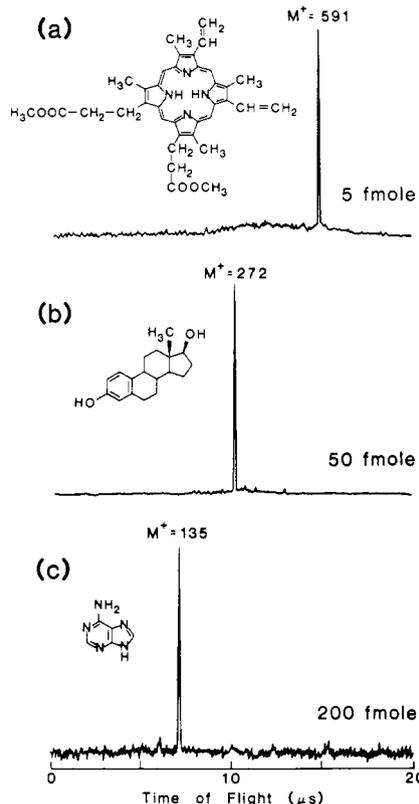
Figure 1. Laser desorption/multiphoton ionization mass spectra of (a) protoporphyrin IX dimethyl ester, (b)  $\beta$ -estradiol, and (c) adenine. The amount of each sample desorbed by a  $\text{CO}_2$  laser pulse is 5, 50, and 200 fmol, respectively. Operating conditions:  $\text{CO}_2$  laser fluence  $\sim 400$   $\text{mJ}/\text{cm}^2$ , Nd:YAG laser fluence  $\sim 3$   $\text{mJ}/\text{cm}^2$ , duty cycle = 10 Hz, and signal averaging time = 20 s.
