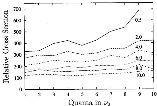
FIG. 2. Relative reaction cross sections (arbitrary units) for the formation of  $\text{NH}_3\text{D}^+$  (deuterium abstraction) as a function of ammonia-ion vibrational state (quanta in  $\nu_2$ ) for center-of-mass collision energies from 0.5 to 10.0 eV. The vibrational spacing is 0.12 eV, so the internal energy spanned by the plot is from 0.12 to 1.2 eV. Each curve represents the average of at least three experiments.
