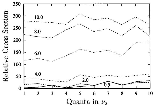
FIG. 5. Relative reaction cross sections (arbitrary units) for the formation of  $\text{CD}_3^+$  (dissociative charge transfer) as a function of ammonia-ion vibrational state (quanta in  $\nu_2$ ) for center-of-mass collision energies from 0.5 to 10.0 eV. The vibrational spacing is 0.12 eV, so the internal energy spanned by the plot is from 0.12 to 1.2 eV. Each curve represents the average of at least three experiments.
