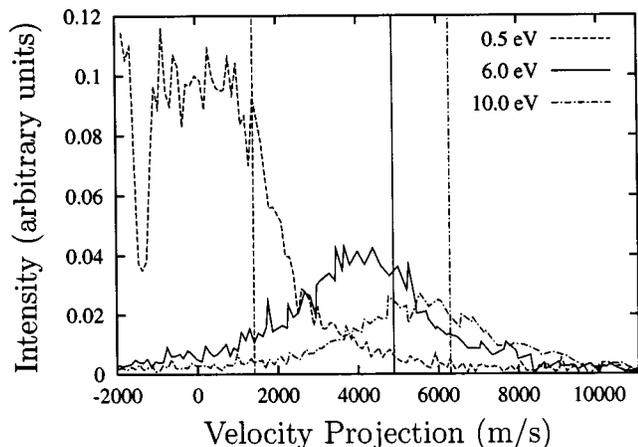
FIG. 4. Center-of-mass frame velocity histograms for  $\text{NH}_3\text{D}^+$  as a function of collision energy. Each curve represents the binned (100 m/s) average of 16 experiments. The vertical lines indicate the prediction of the spectator-stripping assumption.
