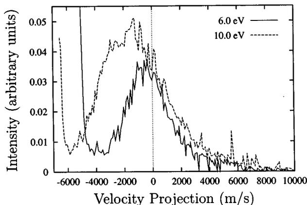
FIG. 6. Center-of-mass frame velocity histograms for  $\text{CD}_3^+$  as a function of collision energy. Each curve represents the average of 33 experiments.
