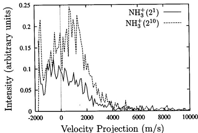
FIG. 3. Center-of-mass frame velocity histograms for  $\text{NH}_3\text{D}^+$  coming from reactions with  $\text{NH}_3^+(2^1)$  and  $\text{NH}_3^+(2^{10})$ . The collision energy is 0.5 eV (com) for both curves. Each curve represents the binned (100 m/s) average of three experiments.
