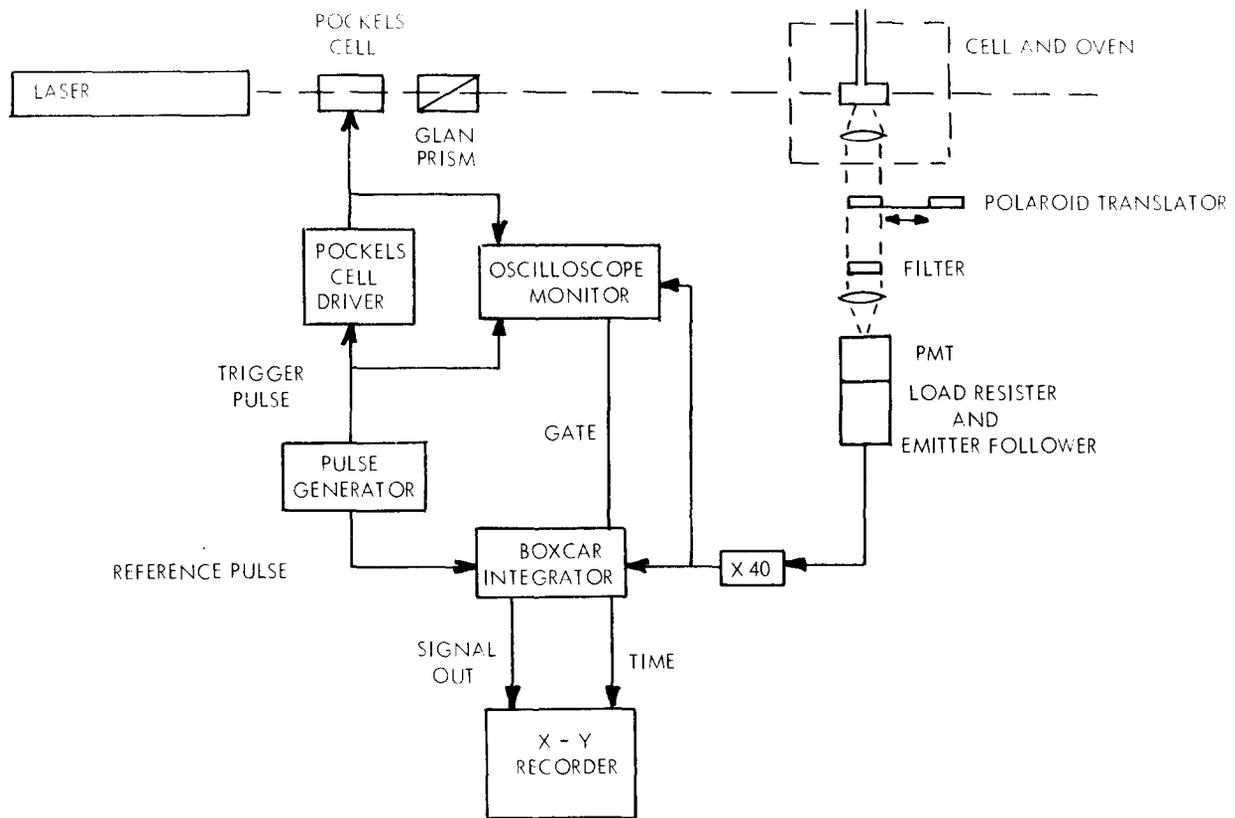
FIG. 3. Experimental setup for the measurement of the time response of a pumped system to the onset of pumping radiation.
