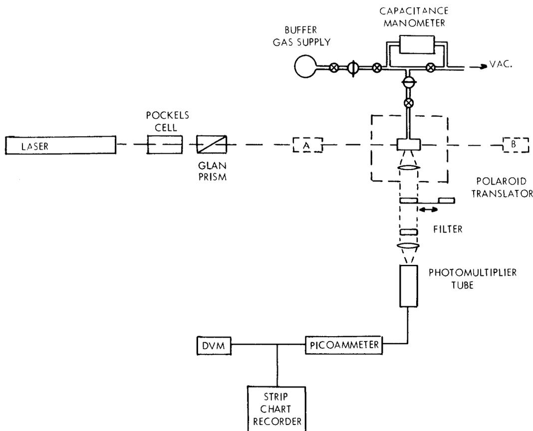
FIG. 1. Experimental setup for the measurement of the steady state degree of polarization as a function of foreign gas pressure.
