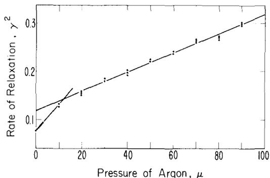
FIG. 6. Plot of the pumping parameter,  $\gamma^2$ , as a function of argon pressure.
