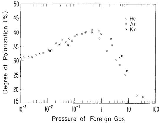
FIG. 4. Steady state degree of polarization as a function of foreign gas pressure (torr).
