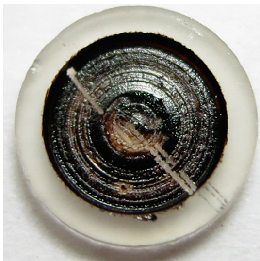
Figure 2. Photograph of the asphaltene sample platter after L 2 MS measurement. The laser desorption process desorbs essentially all asphaltenes from the area where the laser strikes the sample (white diagonal lines).
