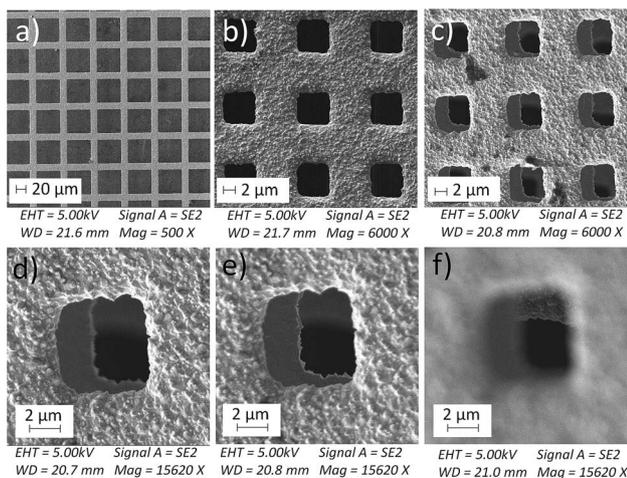
Fig. 4 Scanning electron microscopy (SEM) images of meshes with sizes of (a) 50  $\mu\text{m}$ , (b) 5.5  $\mu\text{m}$ , and (c) three layers of 5.5  $\mu\text{m}$  mounted in front of the microdroplet spray nozzle; (d), (e), and (f) show the focus on the first, second and third layer of meshes used in (c).
