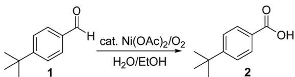
Scheme 1 Oxidation of 4-*tert*-butylbenzaldehyde **1** with molecular oxygen and 5 mol% Ni(OAc)<sub>2</sub> in water–ethanol (*v/v* = 1 : 1.2) to form 4-*tert*-butylbenzoic acid **2**.
