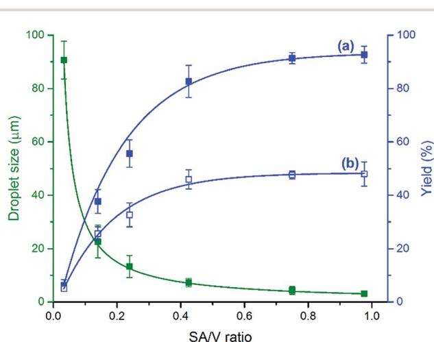
Fig. 3 Dependence of product yield on the SA/V ratio in microdroplet aerobic oxidation of 4-*tert*-butylbenzaldehyde to 4-*tert*-butylbenzoic acid: (a) using O<sub>2</sub> as the oxidant; and (b) using air as the oxidant.
