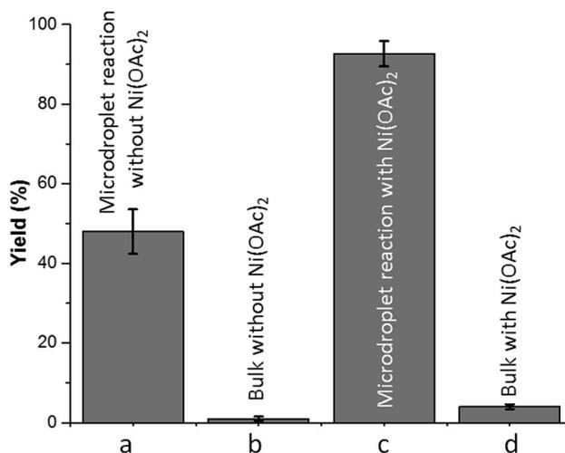
Fig. 2 Oxidation of 4-*tert*-butylbenzaldehyde **1** with molecular oxygen in water–ethanol (*v/v* = 1 : 1.2): (a) in microdroplets without adding Ni(OAc)<sub>2</sub>; (b) in bulk without adding Ni(OAc)<sub>2</sub>; (c) in microdroplets with 5 mol% Ni(OAc)<sub>2</sub>; and (d) in bulk with 5 mol% Ni(OAc)<sub>2</sub>. The collection time for droplet reaction is 30 min and the bulk-phase reaction time is the same. Error bars represent one standard deviation (3 measurements).
