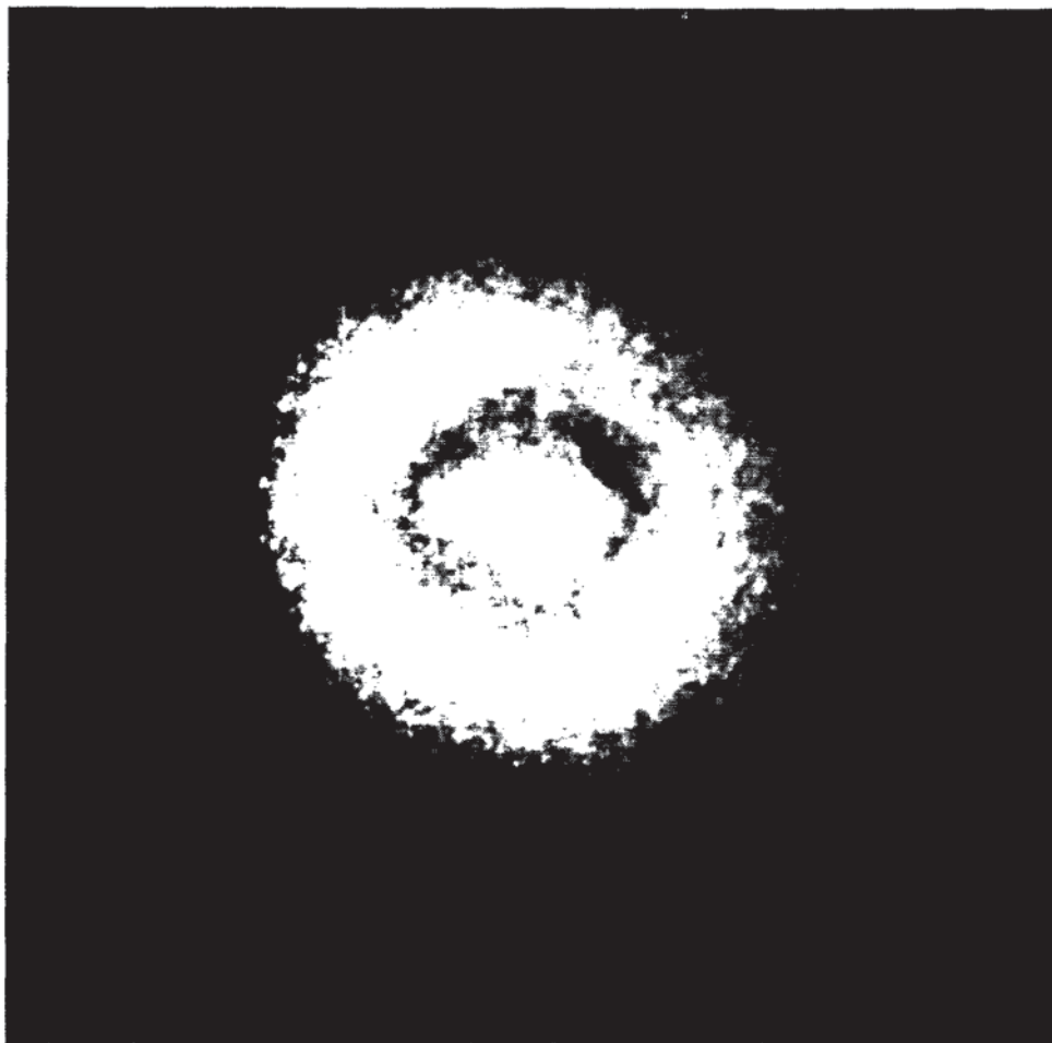
FIG. 2. Ion image of H_2 ( v=1, J=11 ) formed in the reaction H + HI \rightarrow H_2 + I initiated in a beam of neat HI. Fast H atoms are formed by laser photolysis of HI, and the H_2 products are ionized by (2+1) REMPI before being projected onto a position-sensitive detector. The ion density is represented by a continuous grey scale (white being highest intensity).
