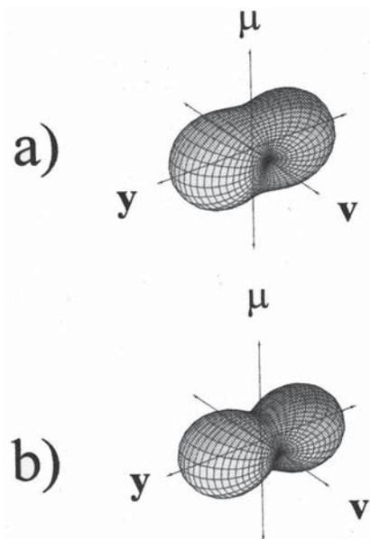
FIG. 8. (a) Plots of the Cl-photofragment angular momentum distributions from the photodissociation of  $\text{Cl}_2$  at 320 nm. Notice that the  $J=3/2$  angular momentum is strongly peaked perpendicular to both the recoil direction  $\hat{v}$  and the transition dipole moment  $\mu$ . (b) A plot of the  $m_y = \pm 3/2$  distribution, showing the strong similarity with the experimental measurement, and that the measured Cl atoms are nearly maximally aligned with respect to the  $y$  axis.
