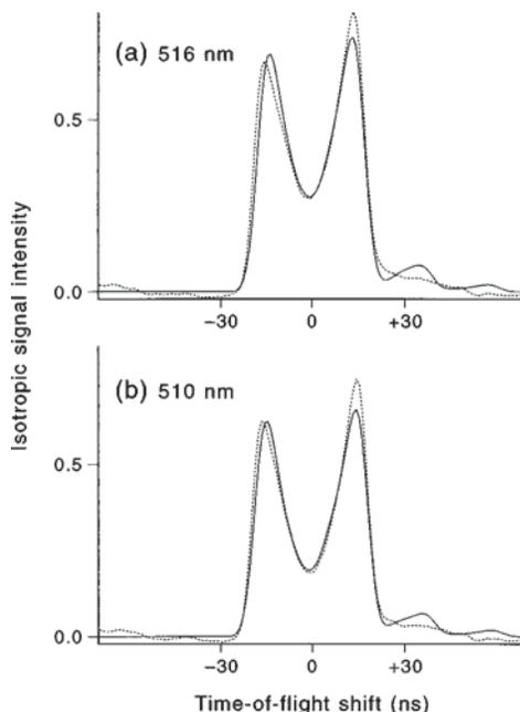
FIG. 4. (a) The isotropic  $^{37}\text{Cl}^+$  ion-arrival composite profile,  $I_{\text{iso}}^Z$ , from the photodissociation of ICl at 516 nm and (b) at 510 nm. Notice that the profiles are very similar; the profile at 510 nm is somewhat more dipped in the center than the profile at 516 nm, as  $\beta$  at this frequency is somewhat more positive. Other than this, there are no large changes in the speed distribution.
