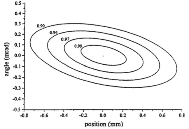
FIG. 2. Acceptance contours for a ring-down cavity of length 2.114 m and mirror radius of curvature 6.0 m. Contours were calculated for normalized stacked energies of 0.99, 0.97, 0.94, and 0.90.
