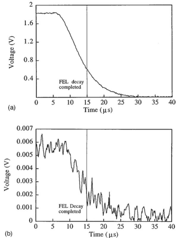
FIG. 5. Single shot ring-down decay waveform obtained with spectrometer slits completely open (a) without pulse stacking, and (b) with pulse stacking.
