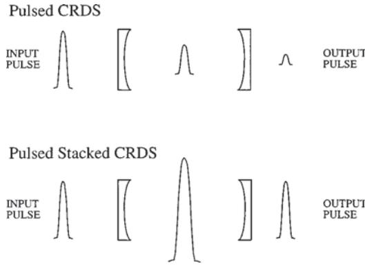
FIG. 1. Illustration of the difference between pulsed CRDS and pulse-stacked CRDS. For cavity mirrors with 500 ppm transmission, the transmitted energy for pulsed CRDS is  $(2.5 \times 10^{-7})U_{\text{inc}}$ . For pulse-stacked CRDS the pulse energy inside the RDC is  $(2 \times 10^3)U_{\text{inc}}$  and the transmitted energy is  $U_{\text{inc}}$ .
