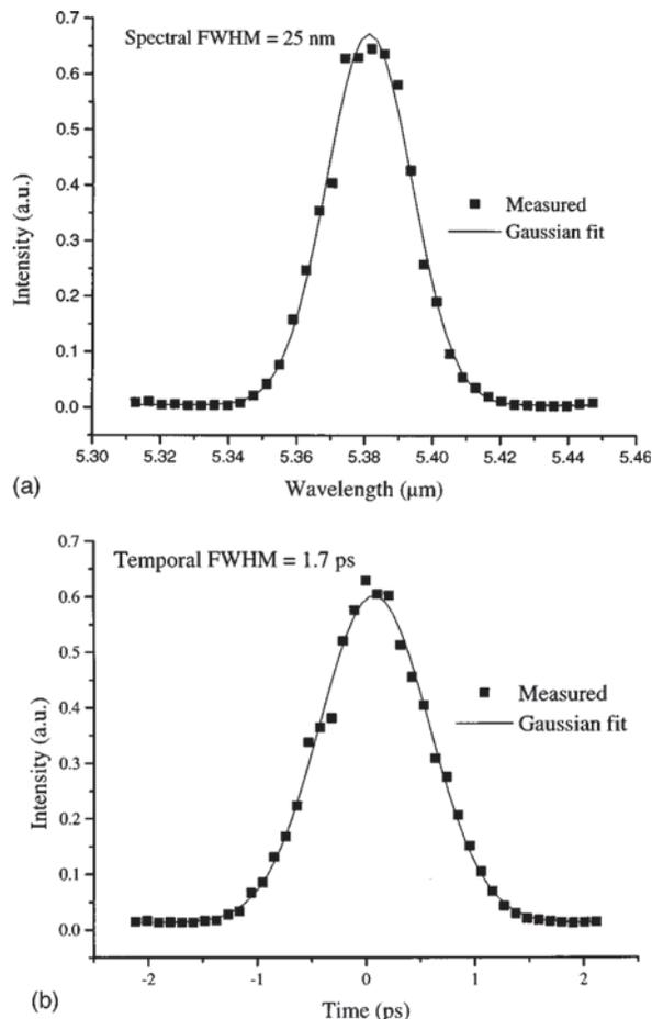
FIG. 3. FEL diagnostics showing (a) laser spectral width, and (b) pulse autocorrelation at  $5.38\ \mu\text{m}$ . The measured  $\Delta f\Delta t$  (FWHM)  $\approx 0.44$ , in agreement with the value calculated for a Gaussian beam.
