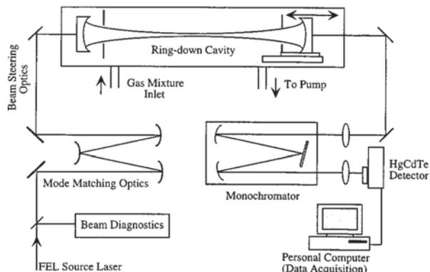
FIG. 4. Experimental setup to perform pulse-stacked cavity ring-down spectroscopy.
