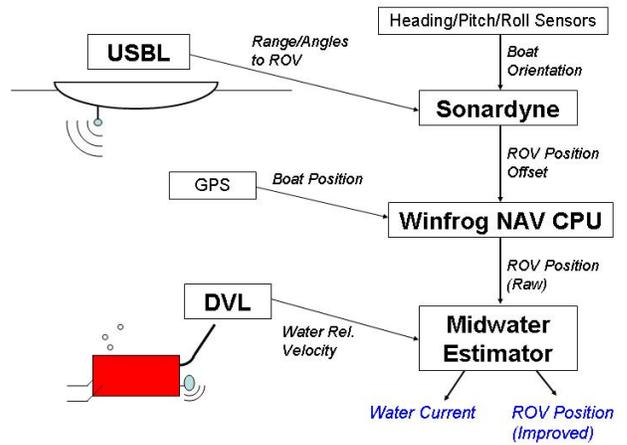
Fig. 8. Block Diagram of System
