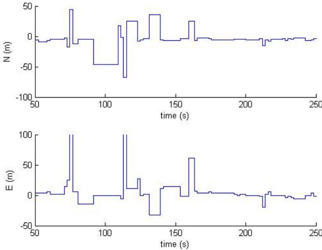
Fig. 2. USBL Jumps due to Cavitation
