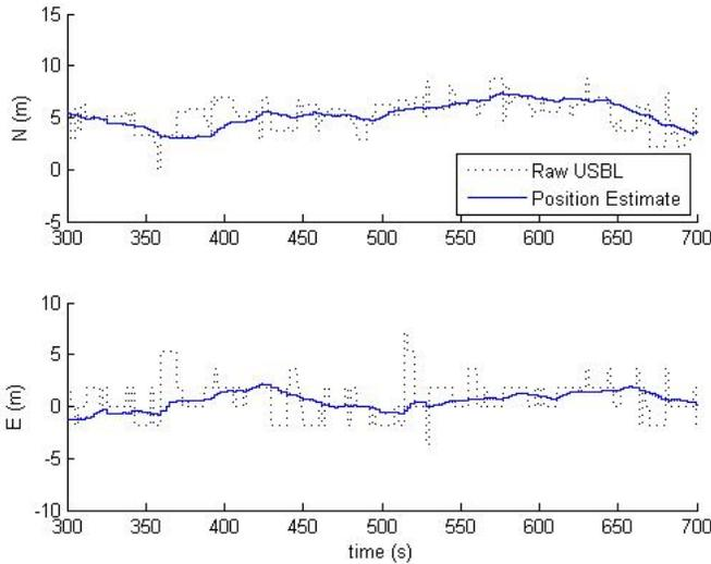
Fig. 10. Position vs. Time (100 m Depth)
