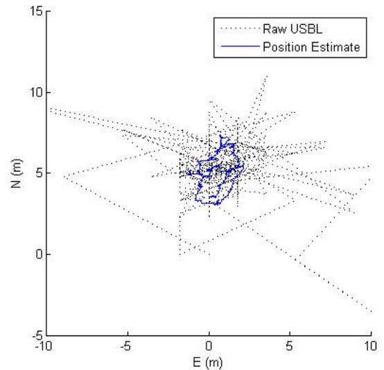
Fig. 9. ROV XY Position Estimate (100 m Depth)
