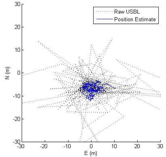
Fig. 12. ROV XY Position Estimate (640 m Depth)
