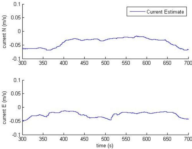
Fig. 11. Current vs. Time (100 m Depth)
