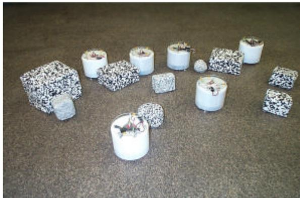
Figure 1: Robots and obstacles from the Micro-Autonomous RoverS (MARS) test platform.
