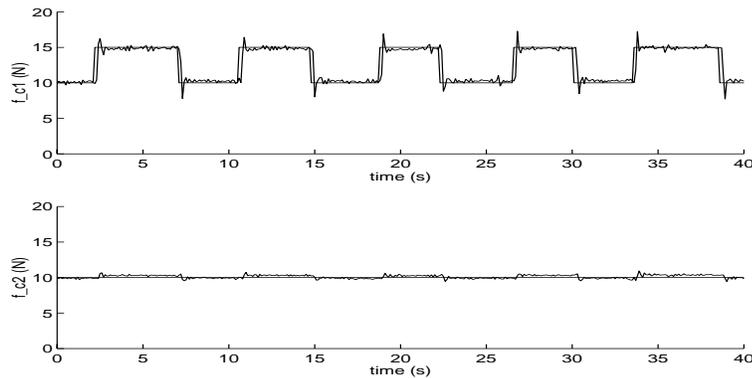
Figure 8. Multi Contact Force Control
