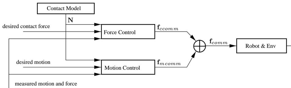
Figure 4. Decoupled Architecture for Force/Motion Control
