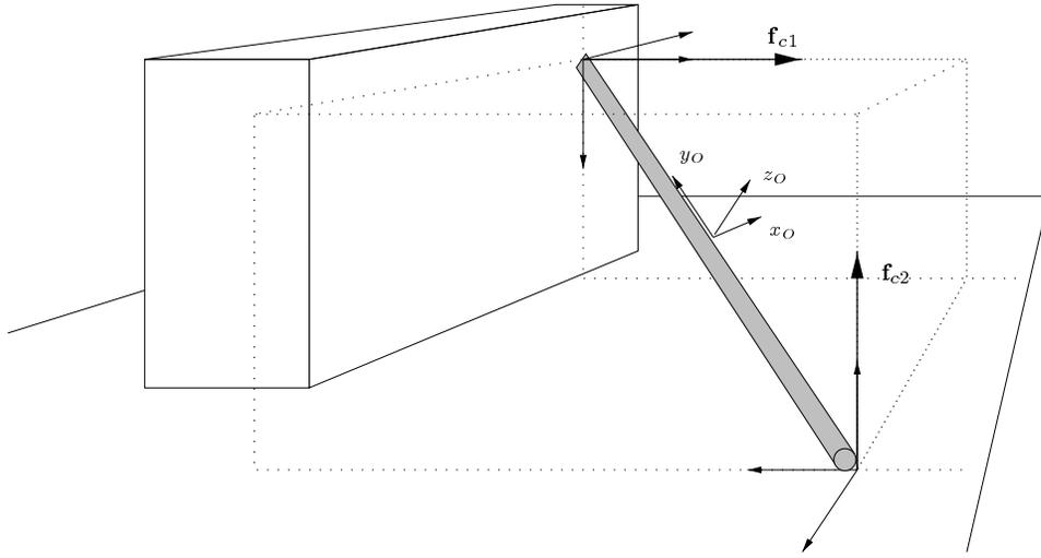
Figure 1. A general two-point contact with skew, non-intersecting contact normals.
