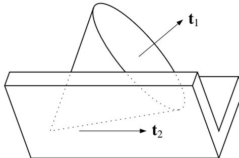
Figure 2. A cone with two motion freedoms: rotation about its axis ( $\mathbf{t}_1$ ) and translation along the groove's axis ( $\mathbf{t}_2$ ). The two axes are neither parallel nor perpendicular.
