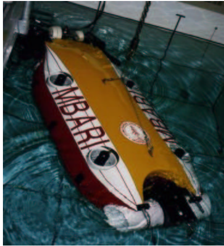
Figure 1.8: OTTER: A Small Underwater Vehicle Operated in MBARI’s Test Tank
