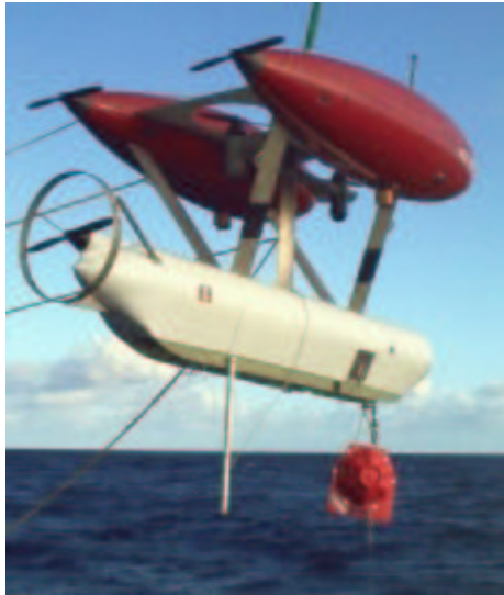
Figure 1.9: Autonomous Benthic Explorer of the Woods Hole Oceanographic Institution [59]
