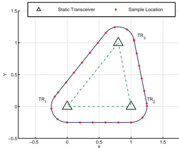
Figure 3: Standard Array Configuration
