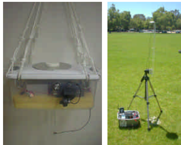
Figure 21: Antenna configuration : an aerial mobile XCVR (left) and a ground-based XCVR (right)
