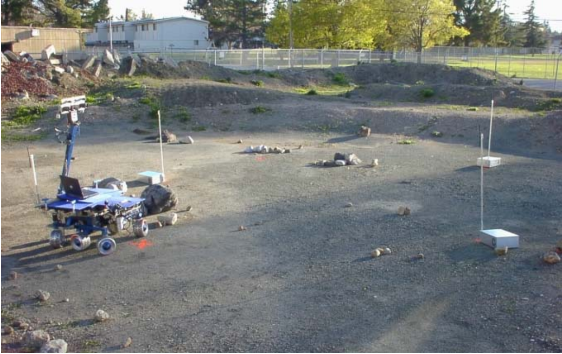
Figure 1: A Self-Calibrating Pseudolite Array (SCPA) deployed over a dry lakebed area in the “Marscape” at the NASA Ames Research Center
