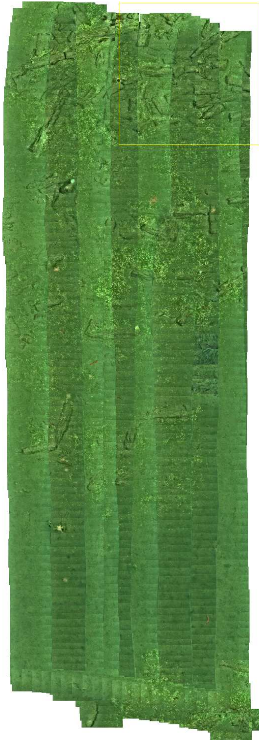
Fig. 4. Portion of a real-time, navigation-grade mosaic of a brachiopod/rubble field in Monterey Bay taken from ROV Ventana , controlled by the real-time mosaicking and navigation system. The camera altitude from bottom was held at 1.8 m. The total area covered was about 13 m \times 72 m, containing 2136 tiles. The mosaic was created without operator input beyond issuing position commands to move the vehicle. This view shows the top half of the surveyed field, covering an area of about 13 m \times 37 m with 1100 tiles.
