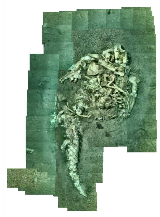
Fig. 1. Navigation-grade mosaic of a whalefall at the bottom of Monterey bay taken from ROV Tiburón . Using the real-time visual mosaicking and navigation system for control, the ROV performed a lawnmower pattern at an altitude between 2.1 m and 3.4 m. The maximum height of the skeleton above the sea floor was about 0.9 m. The mosaic covers an area of about 7 m \times 11 m and contains 120 tiles.
