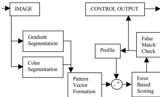
Figure 5. Block Diagram for jelly tracking system.
