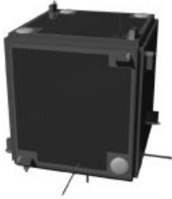
Fig. 1: Orion microsatellite showing the GPS antennas (round) and cold-gas thrusters (at corners).
