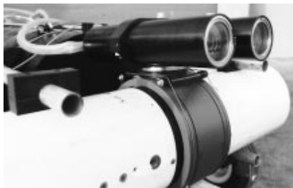
Figure 3: Stereo cameras mounted on a pan/tilt.
