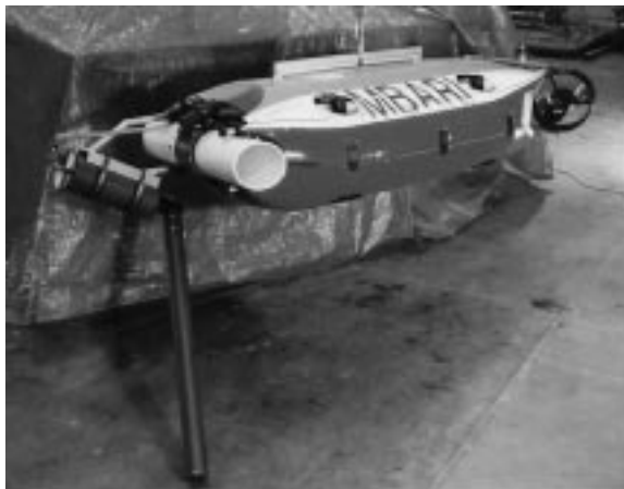
Fig. 12. Single-link manipulator mounted on OTTER .
