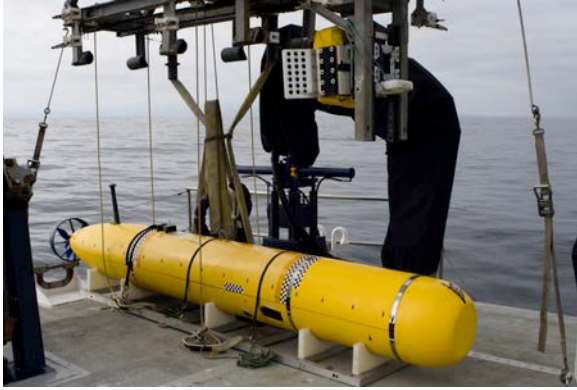
Fig. 2. The MBARI modified Mapping AUV used for the return-to-site tests
