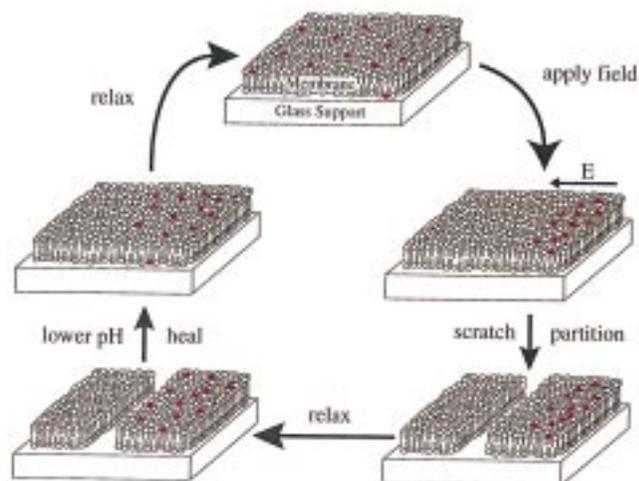
**Figure 2.** Schematic representation of the bilayer partitioning, electrophoresis and healing processes shown in Figure 1.
