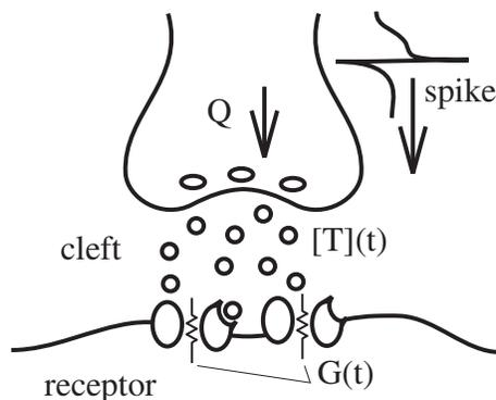
Figure 1.1: The silicon synapse consists of the cleft, which models neurotransmitter concentration,  $[T](t)$ , and the receptor, which models conductance,  $G(t)$ . When a spike arrives it causes an increase in  $[T](t)$ , which bind to receptors increasing  $G(t)$ .
