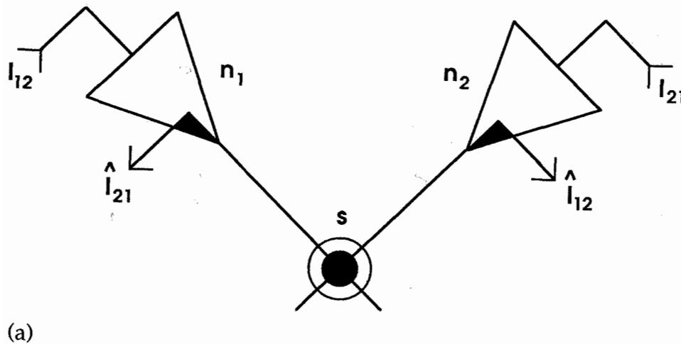
Figure 5: Characteristics of a synthetic neuronal circuit. (a) A simple circuit consisting of two neurons ( $n_1$  and  $n_2$ ) and a synapse ( $s$ ) was built and tested to demonstrate the proposed communication scheme. The currents sent by  $n_1$  ( $n_2$ ) and that received by  $n_2$  ( $n_1$ ) are denoted by  $I_{12}$  ( $I_{21}$ ) and  $\hat{I}_{12}$  ( $\hat{I}_{21}$ ), respectively. Continued on next page.
