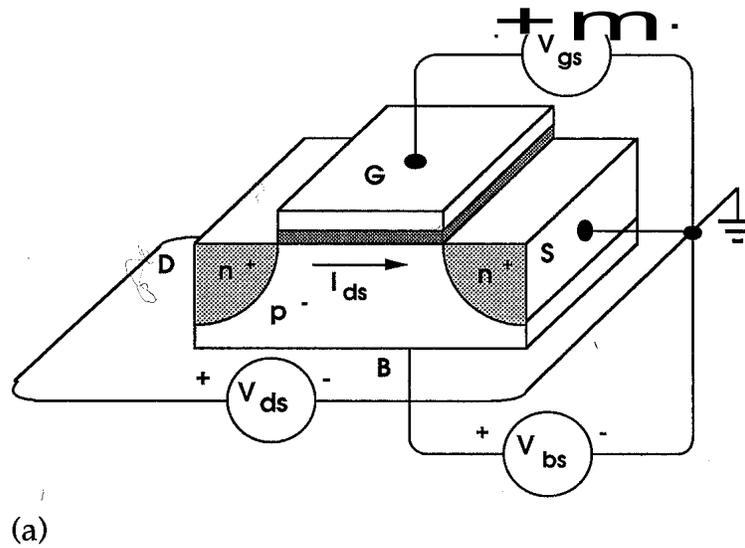
Figure 1: The MOS transistor. (a) Structure.
