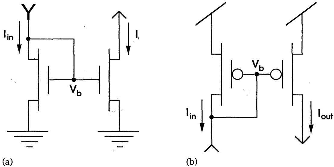
Figure 3: Current mirror circuits using (a) n-type and (b) ptype transistors. These circuits provide an output current that equals the input current if the devices are perfectly matched. For subthreshold operation, we observe variations of about 10%, on average: using  $4 \times 4\mu\text{m}$  devices.
