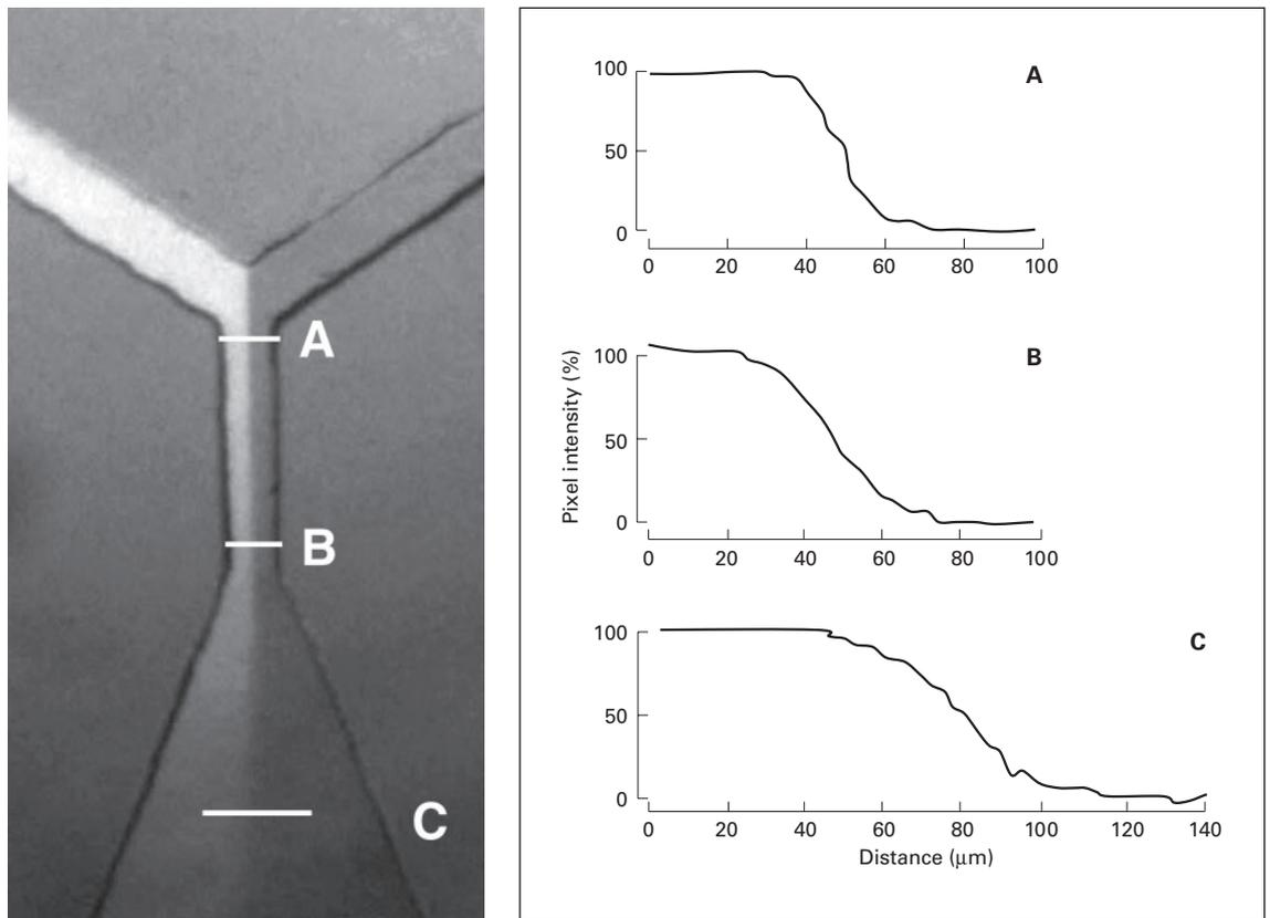
**Fig. 2.** Test of the fluid gradients produced by delivery of a fluorescent dye versus clear fluid to the forced-choice (**A**), free-choice (**B**) and presentation (**C**) regions of the device. A sharp gradient is created in the forced-choice and free-choice regions. A diffuse gradient is created when the microchannel exits into the presentation region, in both the horizontal and vertical dimensions. Adapted from Wittig et al. [2005].
