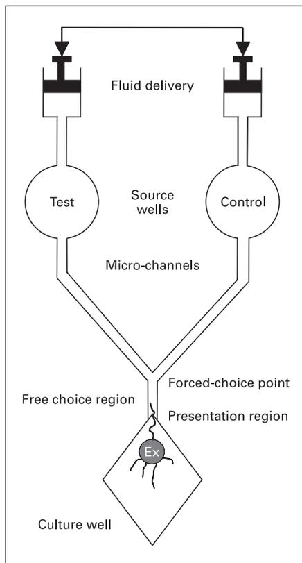
**Fig. 1.** Schematic diagram of a microfluidic device for creation of a fluid gradient and choice point for growing neurites. The device is generated by photolithography and molding. Test and control fluids are forced through a microchannel network at equal rates. They meet at the forced-choice point of a 'Y', and then flow in parallel through a free-choice presentation region to the tissue culture well.
