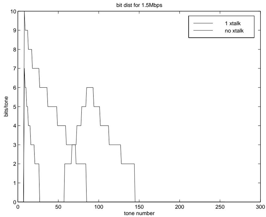
**Figure 2 – Optimized bit distributions for 0 crosstalkers and 1 crosstalker on 4.25 km 26-gauge twisted pair (xtalk is HDSL, background noise is -140 dBm/Hz).**
