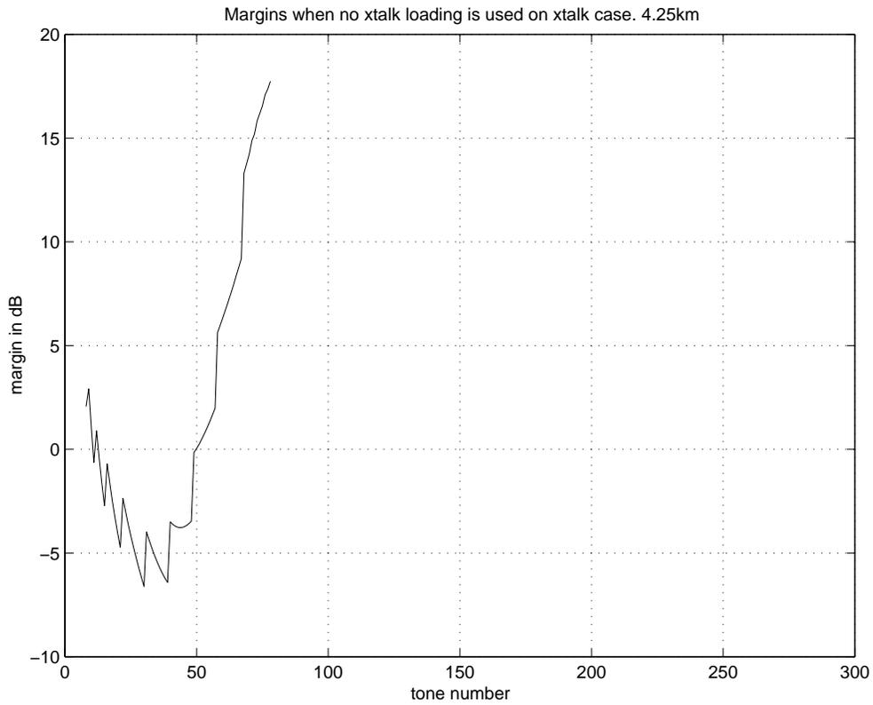
**Figure 3 – Margin for NO SWAPPING when the crosstalker is turned on.**
