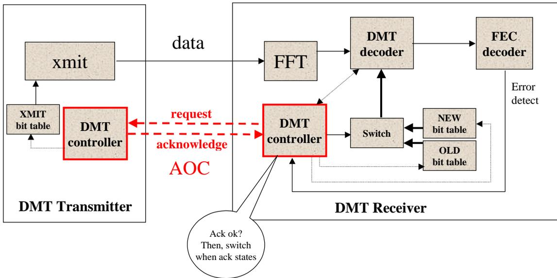
a). Bit swap with AOC functioning properly – Receiver DMT controller switches to new bit table at time specified by AOC acknowledgement.
