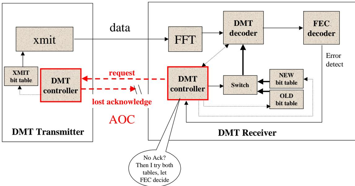
b). Bit swap with lost AOC acknowledgement – Receiver DMT controller tries both switch settings using the FEC decoder correct/errors detect to arbitrate.
