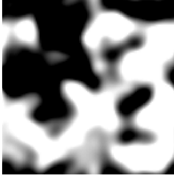
FIGURE 1. Initial distribution of the conserved scalar. White regions denote \xi = 1 while black regions denote \xi = 0 . Initial conserved scalar unmixedness \Omega = 0.84 .
