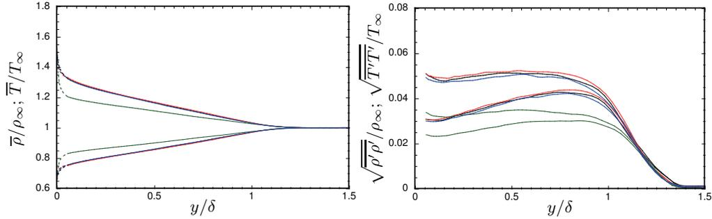
FIGURE 6. Mean and fluctuation density (lower curves) and temperature (upper curves) for outer-layer WMLES. Black, EQBL; red line, CNST; green, CDYN; blue, VDYN ( $\alpha = 1.2$ ).
