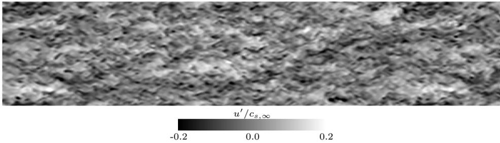
FIGURE 7. Instantaneous streamwise velocity fluctuation in a wall-parallel plane at the matching location ( $y/\delta = 0.056$ ,  $y^+ = 856$ ). The figure covers the full domain, i.e.,  $15 \times 3$  in terms of the boundary layer thickness at the inlet.
