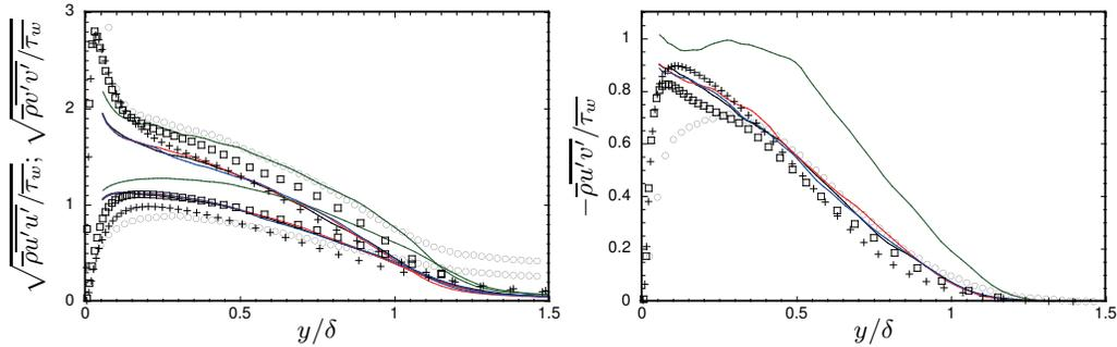
FIGURE 5. Resolved velocity fluctuations (left: upper curves,  $u'$ ; lower curves,  $v'$ ) and Reynolds shear stress (right) for outer-layer WMLES. Black, EQBL; red line, CNST; green, CDYN; blue, VDYN ( $\alpha = 1.2$ ); circles (dual-PIV), experiments (Souverein 2010); squares, DNS at Mach 2.28 and  $Re_\theta \approx 2300$  (Pirozzoli & Bernardini 2010); pluses, incompressible DNS at  $Re_\theta = 900$  (Wu & Moin 2009).
