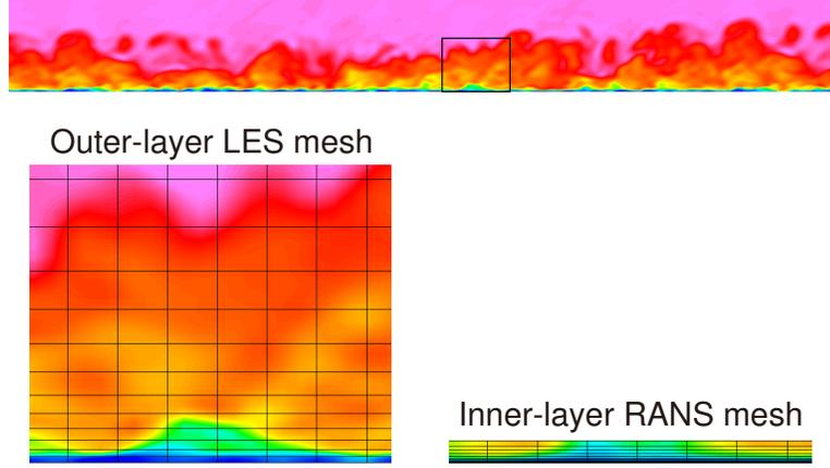
FIGURE 1. Inner-layer RANS and outer-layer LES meshes.
