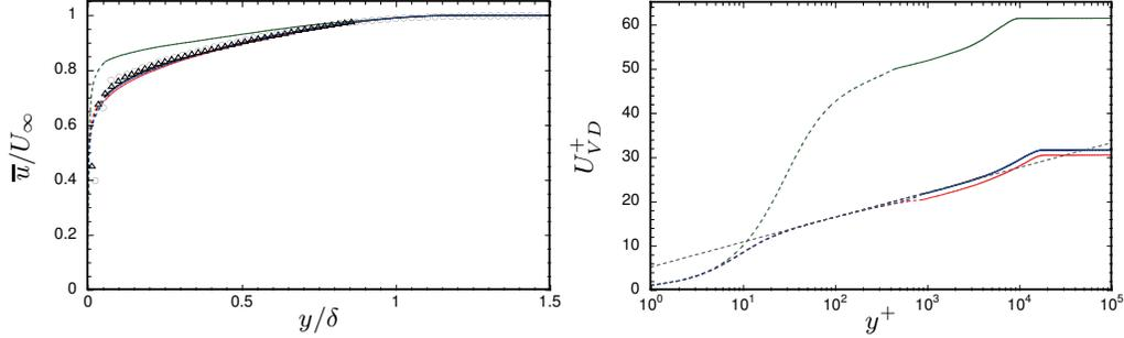
FIGURE 3. Mean streamwise velocity profiles:  $\delta$  scaling on left and Van Driest scaling on right. EQBL (black), CNST (red, lowest curve), CDYN (green, uppermost curve), VDYN with  $\alpha = 1.2$  (blue), Log-law  $U_{VD}^+ = 1/0.41 \log(y^+) + 5.2$  (dashed). Symbols (circles, dual-PIV; triangles, high-resolution zoom-PIV), experiments by (Souverein 2010). Solid lines, outer-layer WMLES; dashed lines, inner-layer RANS.
