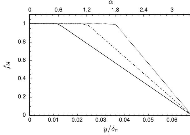
FIGURE 2. Linear blending function  $f_{bl}$ . Solid line,  $\alpha = 0.6$ ; dashed-dotted line,  $\alpha = 1.2$ ; dotted line,  $\alpha = 1.8$ .
