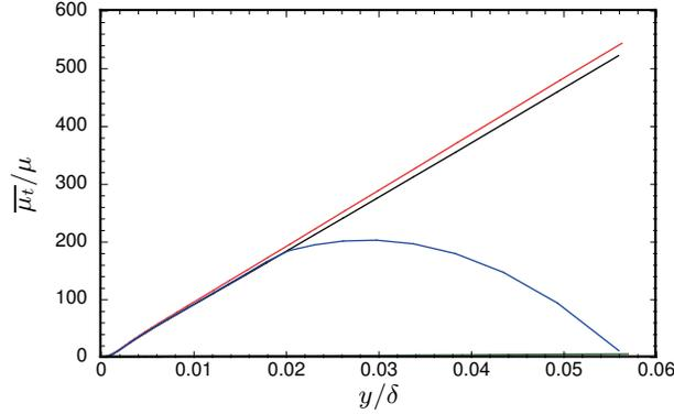
FIGURE 4. Mean turbulent eddy viscosity in inner-layer RANS. EQBL (black), CNST (red, uppermost curve), CDYN (green, close to horizontal axis), VDYN with  $\alpha = 1.2$  (blue, curved shape).
