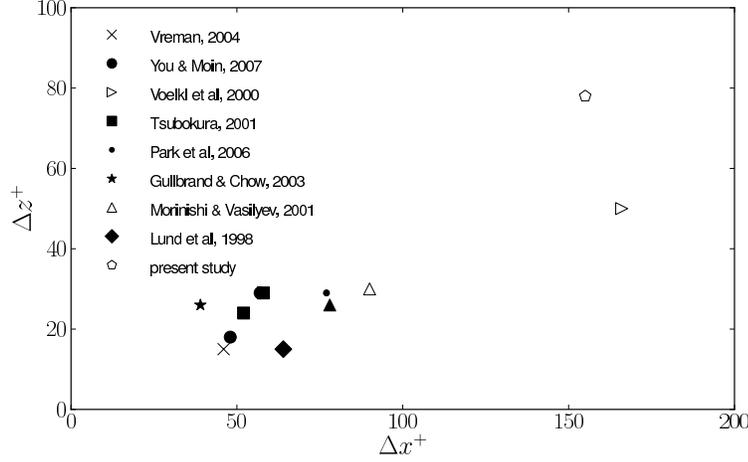
FIGURE 1. Streamwise ( $\Delta x^+$ ) and spanwise ( $\Delta z^+$ ) resolutions for small survey of wall bounded LES calculations where the performance of the subfilter/subgrid scale model was investigated. Open symbols denote simulations for  $Re_\tau > 1000$  and closed symbols denote simulations for  $Re_\tau < 1000$ .
