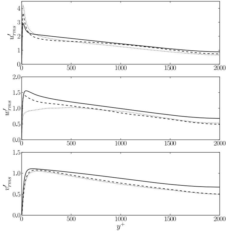
FIGURE 5. Estimation of unfiltered rms velocity fluctuations for the dynamic mixed  $k|\bar{S}|^{-1}$  (---) and dynamic mixed Vreman ( $\cdots$ ) compared to DNS (Hoyas & Jiménez 2006) (—).
