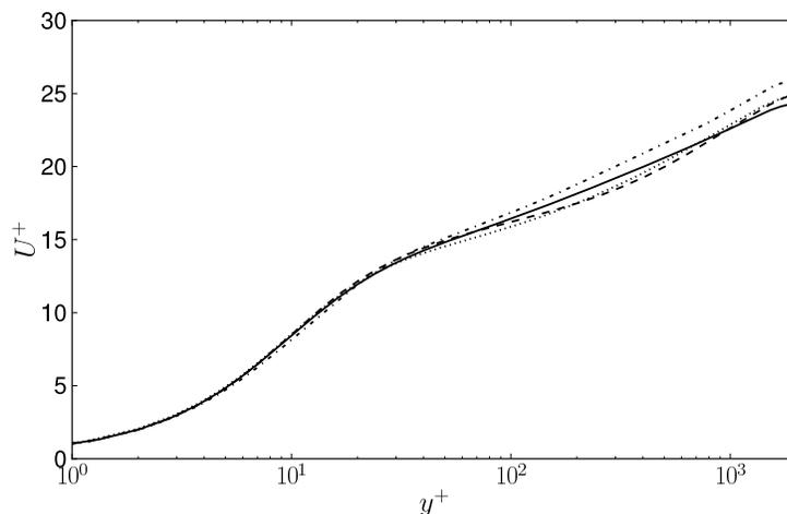
FIGURE 3. Streamwise mean velocity profile for a turbulent channel flow at  $Re_\tau = 2000$  using the dynamic mixed Smagorinsky ( $-\cdot-$ ), dynamic mixed  $k|\bar{S}|^{-1}$  ( $- -$ ), and dynamic mixed Vreman ( $\cdots$ ) models compared with the filtered DNS of Hoyas & Jiménez (2006) ( $-$ ).
