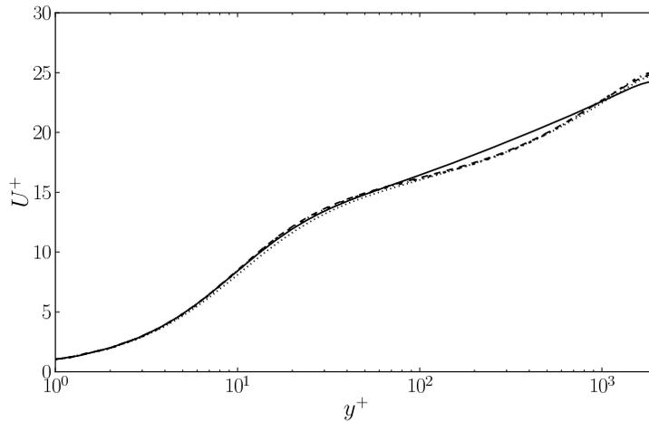
FIGURE 7. Streamwise mean velocity profile for the dynamic mixed  $k|\bar{S}|^{-1}$  model using the  $k$  surrogate defined in Eq. 3.4 (· · ·), Eq. 3.5 (— · —), and Eq. 3.6 (— · —) compared with the filtered DNS of Hoyas & Jiménez (2006).
