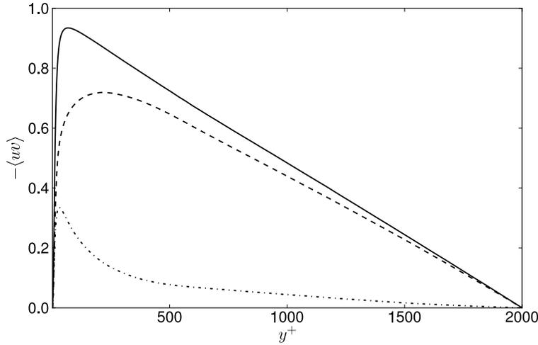
FIGURE 6. Reynolds shear stress contributions from the resolved scales (· · ·), the subfilter stress model (— · —), and their total sum (—) for the dynamic mixed  $k|\bar{S}|^{-1}$  model.
