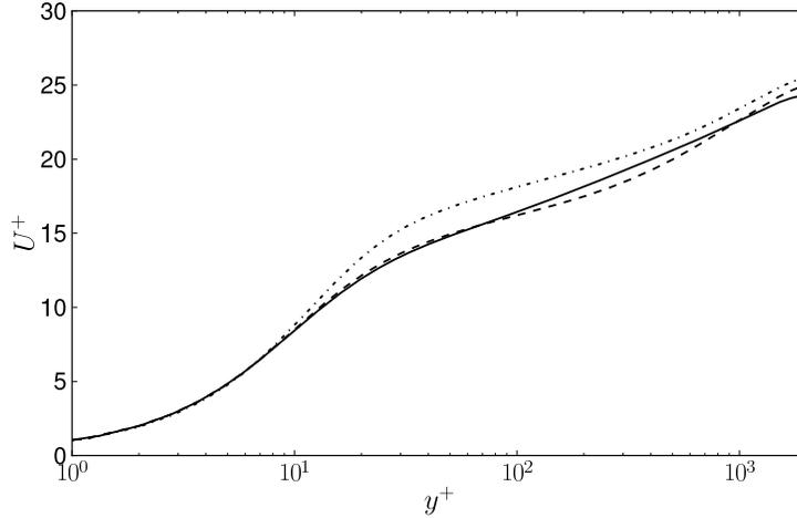
FIGURE 2. Streamwise mean velocity profile for a turbulent channel flow at  $Re_\tau = 2000$  using the dynamic Smagorinsky model ( $- \cdot -$ ) and the dynamic mixed  $k|\bar{S}|^{-1}$  model ( $- -$ ) compared with the filtered DNS of Hoyas & Jiménez (2006) ( $-$ ).
