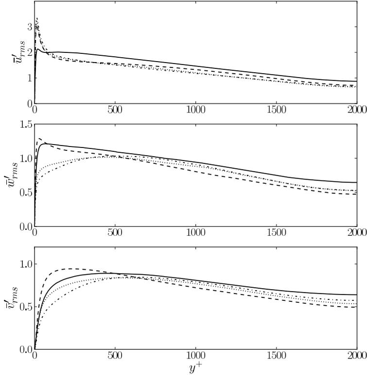
FIGURE 4. Rms velocity profiles for the filtered velocity field for the dynamic mixed Smagorinsky (— · —), dynamic mixed  $k|\bar{S}|^{-1}$  (— —), and dynamic mixed Vreman (· · ·) compared to the filtered DNS of Hoyas & Jiménez (2006) (—).
