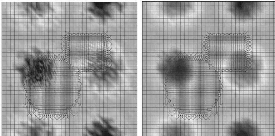
FIGURE 1. A sinusoidal function with superimposed random noise (20% amplitude) on an unstructured grid with two regions of local grid refinement unfiltered (left) and filtered (right).
