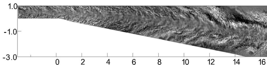
FIGURE 10. Instantaneous spanwise velocity from the LES of the 3D diffuser of Kolade (2010) at  $z/H \approx 1.67$ . Contours are from  $-0.2U_b$  to  $0.2U_b$ .
