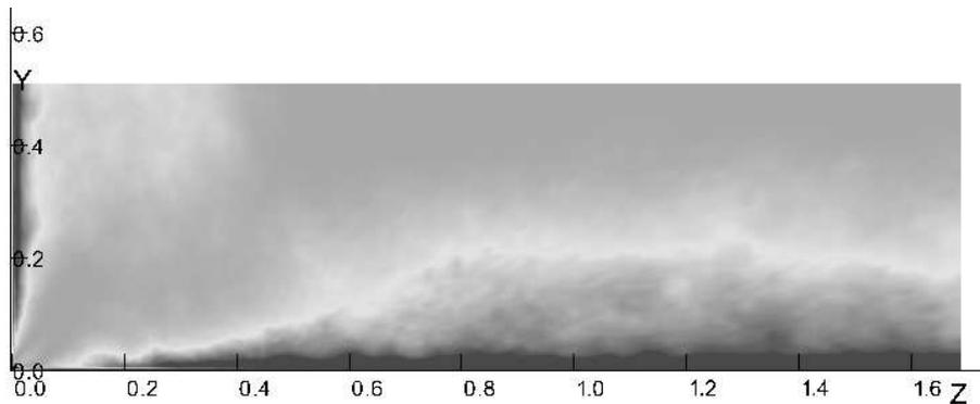
FIGURE 2. Mean contours ( $1 \times 10^{-5}$  to  $1 \times 10^{-3}$ ; log-scale) of  $k^*$  in the bottom left quadrant in a simulation of a rectangular duct flow. Cells that exceeded  $u^* = 0.03$  were subsequently refined.
