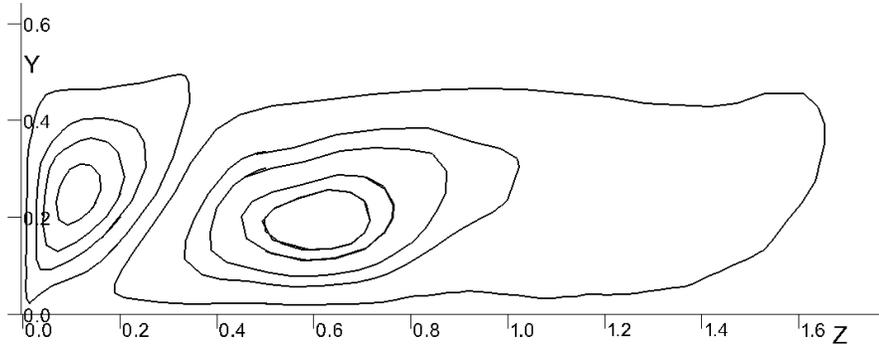
FIGURE 8. Streamlines of the secondary mean velocity vector,  $\vec{U} = (0, V, W)$ , in the bottom left quadrant of the  $yz$  plane in a rectangular duct with aspect ratio 3.33.
