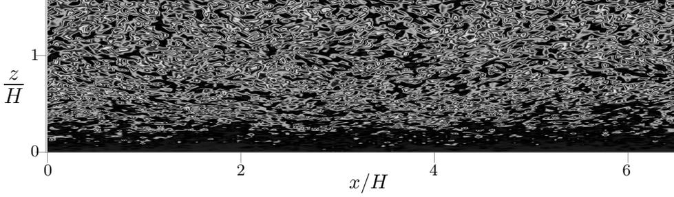
FIGURE 6. Instantaneous values of  $|\tau^{od}| = \sqrt{\tau_{12}^2 + \tau_{13}^2 + \tau_{23}^2}$  in an  $x - z$  plane at  $y/H = 0.025$  (half of the duct span and half of the duct length shown). Contour levels are from 0,  $0.05U_b^2$ .
