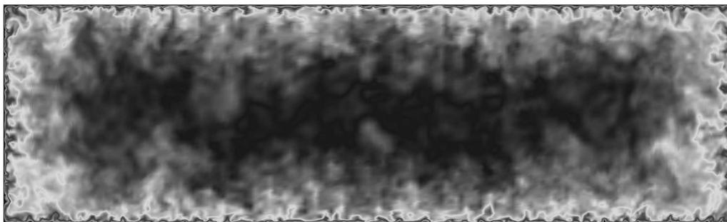
FIGURE 3. Instantaneous streamwise velocity in the  $yz$  plane in a rectangular duct with cross section of  $3.33H \times H$ ; contour levels are from 0 to  $1.4U_b$ .
