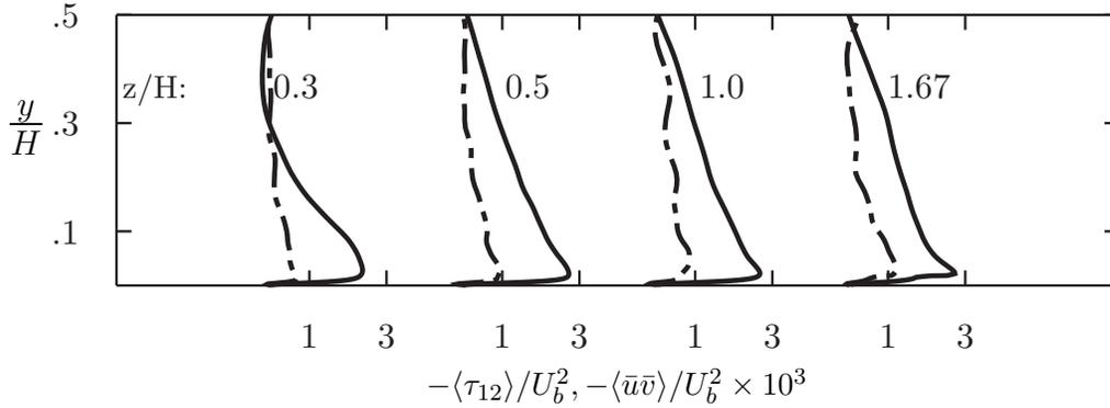
FIGURE 7. Mean profiles of the  $uv$  Reynolds shear stress decomposed into contributions from the resolved scales (—) and the SGS model (---) at different spanwise locations.
