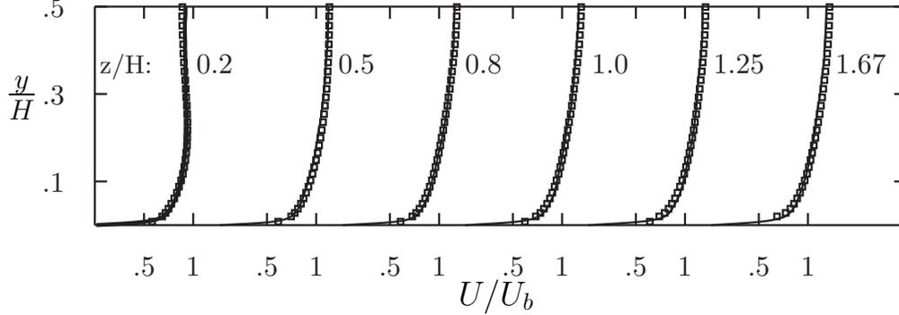
FIGURE 4. Mean streamwise velocity profiles at different spanwise locations for the explicitly filtered LES (solid lines) and the experimental measurements of Kolade (2010) (symbols).
