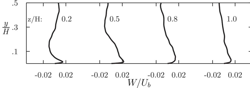
FIGURE 5. Mean spanwise velocity profiles at different spanwise locations for the explicitly filtered LES.
