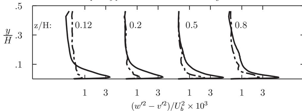
FIGURE 9. Mean profiles of the normal stress anisotropy,  $(w'^2 - v'^2)/U_b^2$ , decomposed into contributions from the resolved scales (—) and the SGS model (---) at different spanwise locations.
