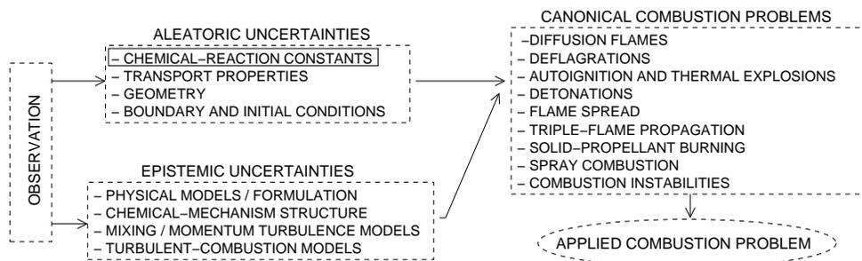
FIGURE 1. Road-map schematics of uncertainty quantification in combustion systems. The present study only tackles the problem of observation-based statistical inference of aleatoric uncertainties in chemical-reaction rates, as indicated by the solid-line rectangle.
