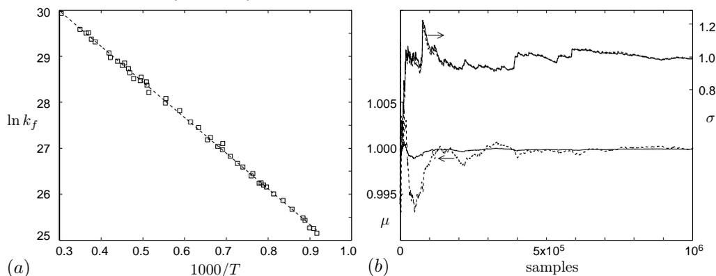
FIGURE 2. (a) Least-squares fit approximation (dashed line) of experimental data of Hong *et al.* (2011*b*) (squares). (b) Convergence of the normalized first and second statistical moments for  $\ln A$  (solid lines) and  $E_a$  (dashed lines)
