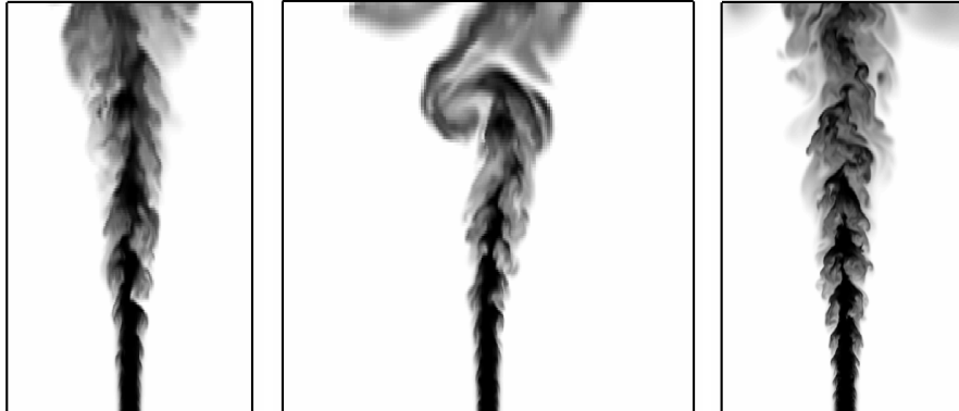
FIGURE 2. Mixture fraction ( Z ) contours, ranging from 0.0 (white) to 1.0 (black). Left: 1 million cell LES with narrow domain; Center: 1 million cell LES with wider domain; Right: 23 million cell mesh with narrow domain.
