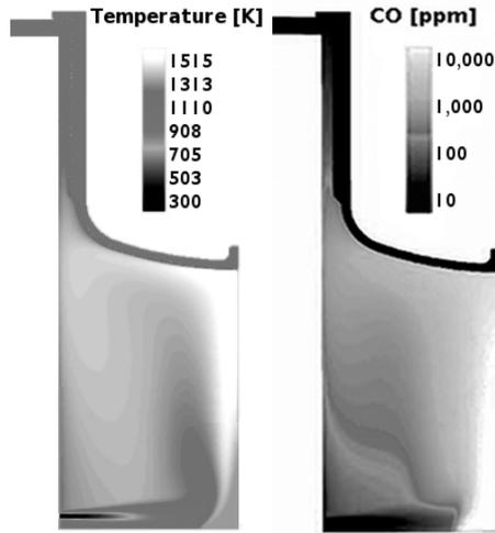
FIGURE 2. Schematic of the case 1 RANS combustion chamber simulation. Left: temperature. Right: CO mole fraction.
