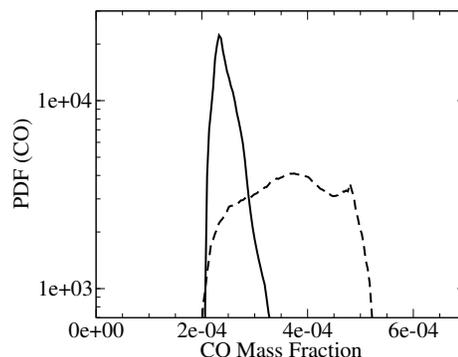
FIGURE 6. Time averaged PDFs from the LES describing CO distributions at the combustor outlet. Solid line (—): case 1; dashed line (---): case 2.
