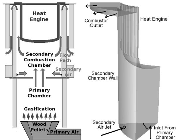
FIGURE 1. Left: schematic of the biomass combustor. Right: schematic of the simulated domain, consisting of a  $1/7^{\text{th}}$  sector of the cylindrical secondary combustion chamber.
