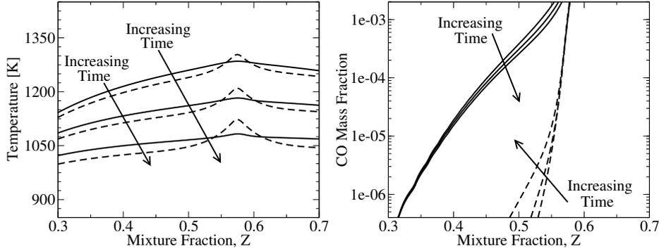
FIGURE 4. CO and temperature from case 1 unsteady flamelets solved using the same  $\chi_{Z,ref}$ . Solid lines (—):  $\alpha = 1 \times 10^1 \text{ K}^{-1} \text{ s}^{-1}$ ; dashed lines (---):  $\alpha = 1 \times 10^{-2} \text{ K}^{-1} \text{ s}^{-1}$ .
