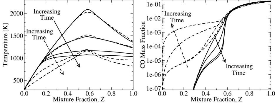
FIGURE 3. CO and temperature from case 1 unsteady flamelets solved using the same heat loss rate  $\dot{q}_L$ . Solid lines (—):  $\chi_{Z,ref} = 1 \times 10^{-3} \text{ s}^{-1}$ ; dashed lines (---):  $\chi_{Z,ref} = 1 \times 10^0 \text{ s}^{-1}$ .
