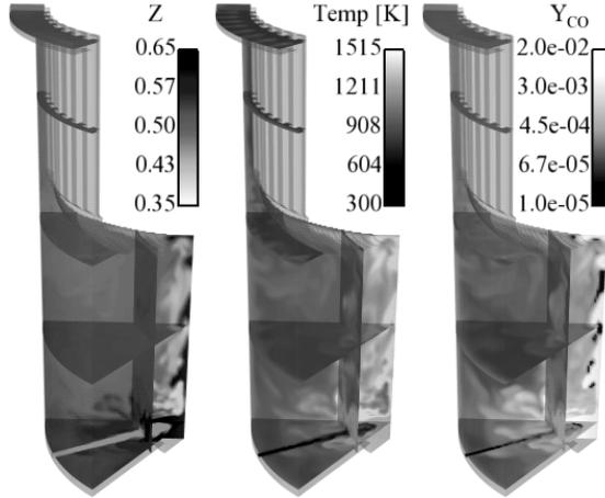
FIGURE 5. Mixture fraction (left), temperature (middle), and CO mass fraction (right) fields in the case 1 LES.
