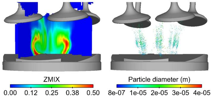
FIGURE 9. Spray injection in engine at 423 CAD. left:mixture fraction; right:spray.
