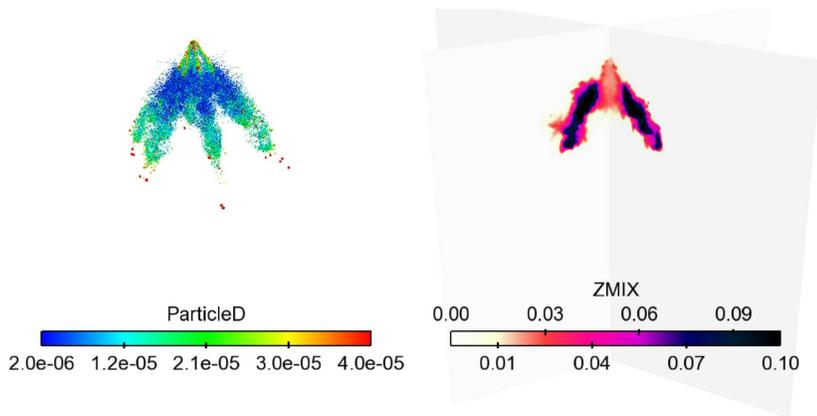
FIGURE 1. Spray particles and the mixture fraction at the start of injection.
