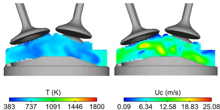
FIGURE 10. Reactive case at 685 CAD. left: temperature; right: velocity.
