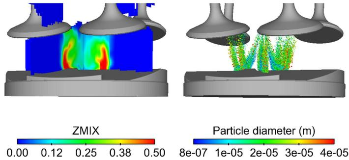
FIGURE 8. Spray injection in engine at 400 CAD. left:mixture fraction; right:spray.
