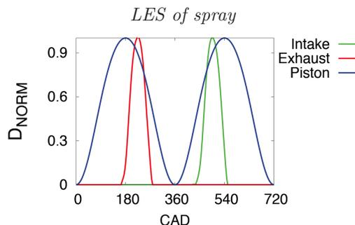
FIGURE 7. Displacement profiles of the piston, intake valve, and exhaust valve against Crank Angle in the engine computation. Source: (Mittal 2012).
