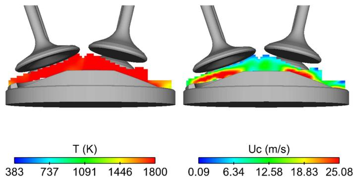
FIGURE 11. Reactive case at 733 CAD. left: temperature; right: velocity.
