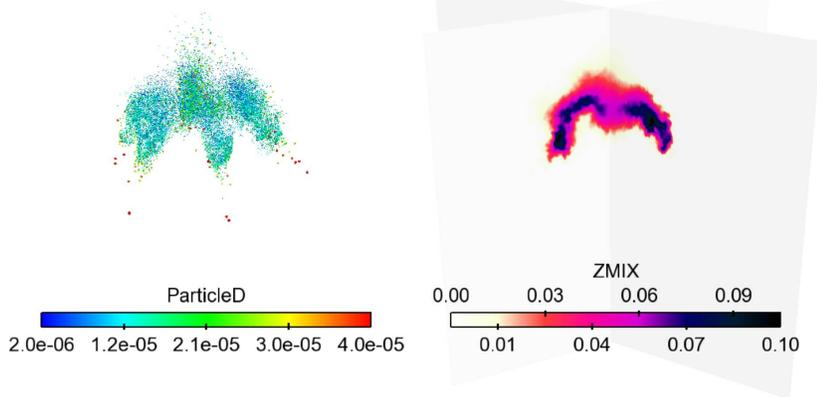
FIGURE 2. Spray particles and the mixture fraction at the end of injection.
