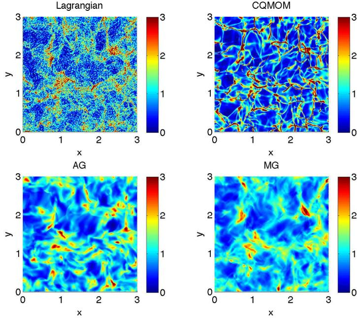
FIGURE 4. Number density for  $St = 20$  from Lagrangian method with 65M particles (top right), CQMOM (top left), AG (bottom left) and MG (bottom right).
