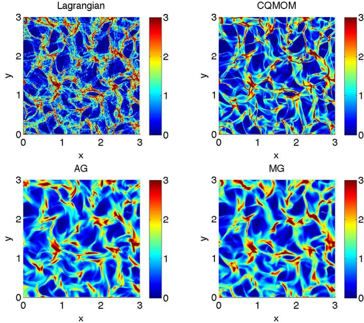
FIGURE 3. Number density for  $St = 5$  from Lagrangian method with 65M particles (top right), CQMOM (top left), AG (bottom left) and MG (bottom right).
