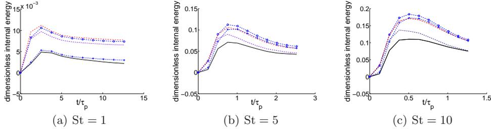
FIGURE 6. Time evolution of phase-average granular temperature from the Lagrangian method projected on a  $256 \times 256$  mesh (black line), CQMOM (violet dashed line), AG (blue dashed line with o), AG with second-order discretization (blue dashed line with +) and MG (red dotted-dashed line).
