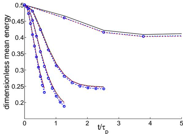
FIGURE 7. Time evolution of phase-average granular energy for  $St = 1, 5, 10$  and  $20$  (top to bottom) from Lagrangian method with 65M particles (black line), CQMOM (green line), AG (blue dots) and MG (red line).
