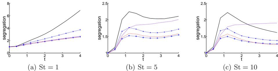
FIGURE 5. Time evolution of mean segregation from the Lagrangian method projected on a  $256 \times 256$  mesh (black line), CQMOM (violet dashed line), AG (blue dashed line with o), AG with second-order discretization (blue dashed line with +) and MG (red dotted-dashed line).
