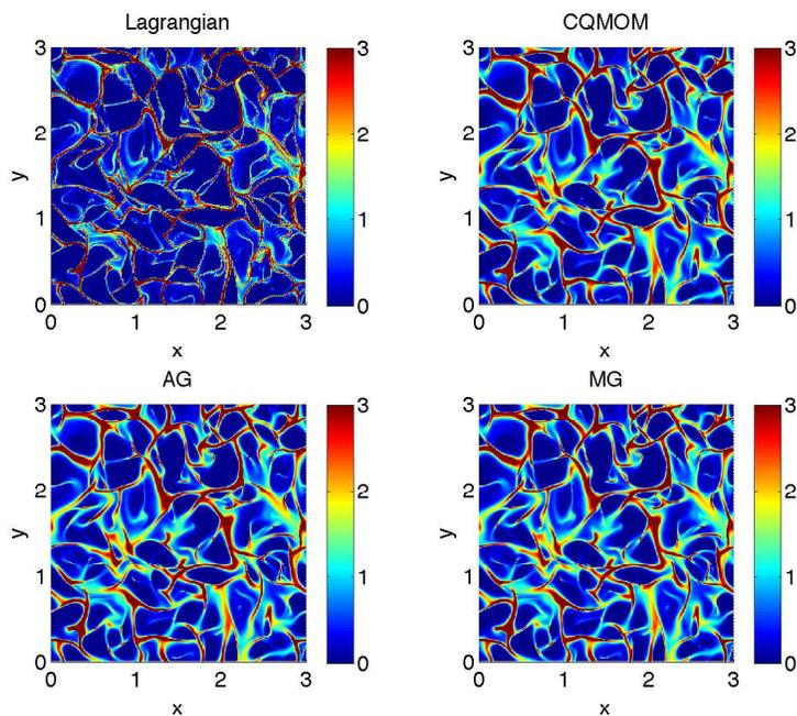
FIGURE 2. Number density for  $St = 1$  from Lagrangian method with 65M particles (top right), CQMOM (top left), AG (bottom left) and MG (bottom right).
