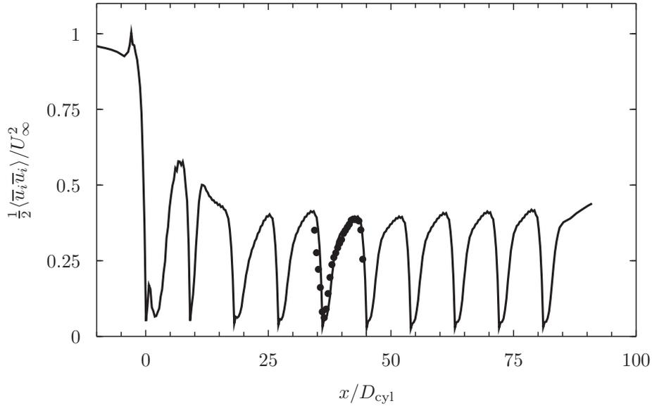
FIGURE 7. Mean kinetic energy behind an array of stationary cylinders (see Figure 6 for precise location of this data) as a function of streamwise coordinate  $x/D$ . The simulation data is the blue line and the experimental data is the black points. The line is the result from the modeled computation and the symbols are from the experiment of Craig *et al.* (2013).
