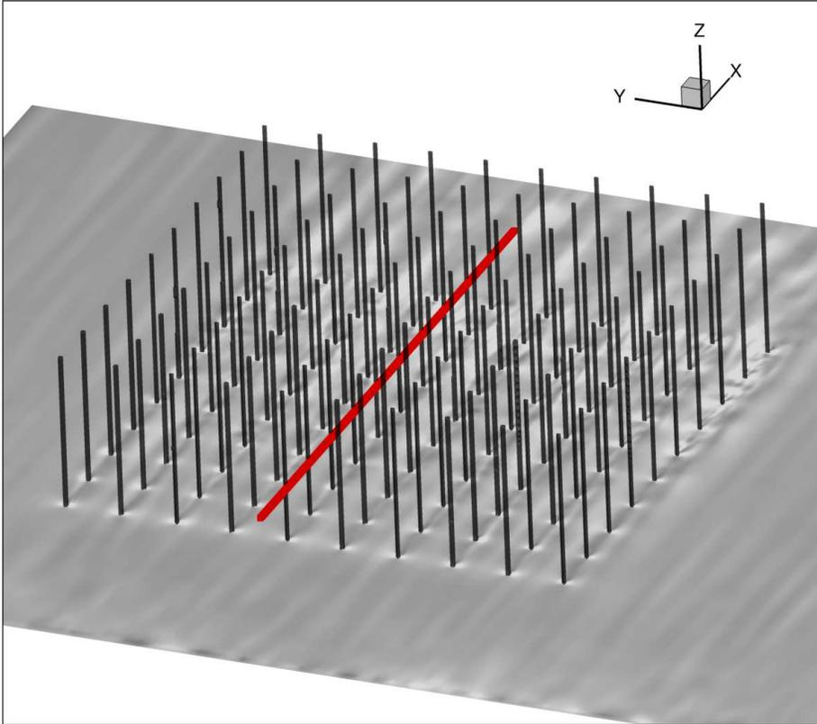
FIGURE 6. Location of data for Figure 7 and 9 (indicated by red line). The data begins ten cylinder diameters upstream of the array  $x/D = -10$  and extends ten cylinder diameters behind the array ( $x/D = 91$ ). The vertical coordinate is kept at  $z/H_{\text{cyl}} = 0.43$ . The spanwise location is immediately behind one of the two center-most cylinders in the array. The line is the result from the modeled computation and the symbols are from the experiment of Craig *et al.* (2013).
