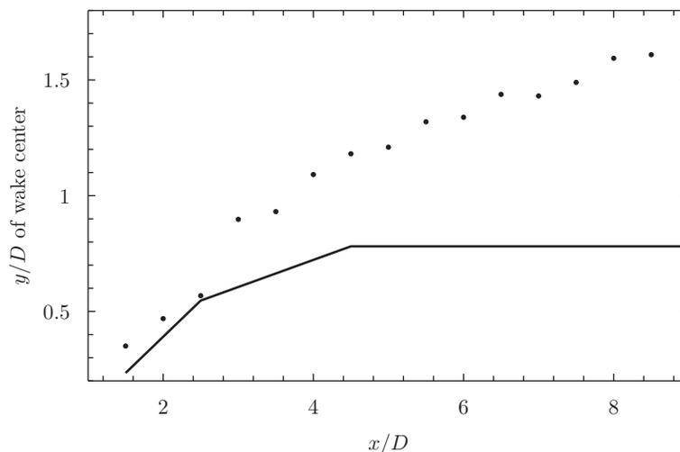
FIGURE 5. Vertical location  $y/D$  of the center of the wake behind a cylinder rotating with  $\hat{\Omega} = 1.5$ , as a function of streamwise coordinate  $x/D$ . The lines are the results for the modeled computation, and the symbols are from our DNS.
