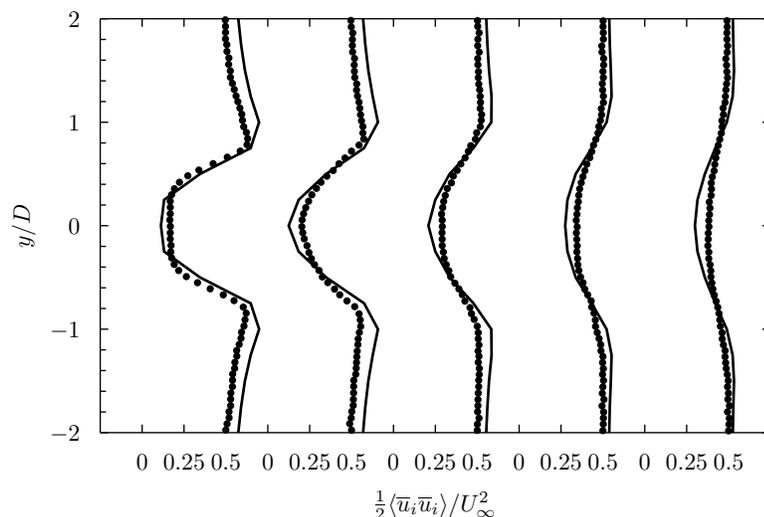
FIGURE 2. Mean kinetic energy profiles,  $\langle \bar{u}_1 \rangle$  as a function of vertical coordinate  $y/D$  at various locations  $x/D = 1.2, 1.5, 2.0, 2.5, 3.0$ , with  $x/D = 0$  corresponding to the cylinder center for a stationary cylinder. The lines are the results for the modeled computation, and the symbols are from the DNS of Mittal & Balachandar (1997).
