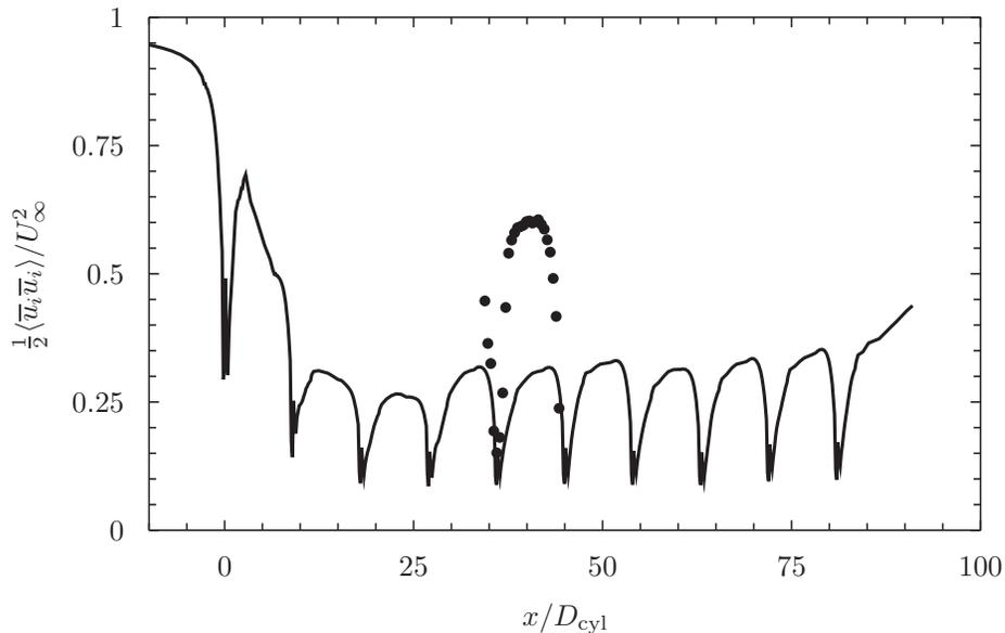
FIGURE 9. Mean kinetic energy behind an array of rotating cylinders ( $\hat{\Omega} = 1.67$ ). See Figure 6 for a more detailed description of data location within the array. The line is the result from the modeled computation and the symbols are from the experiment of Craig *et al.* (2013).
