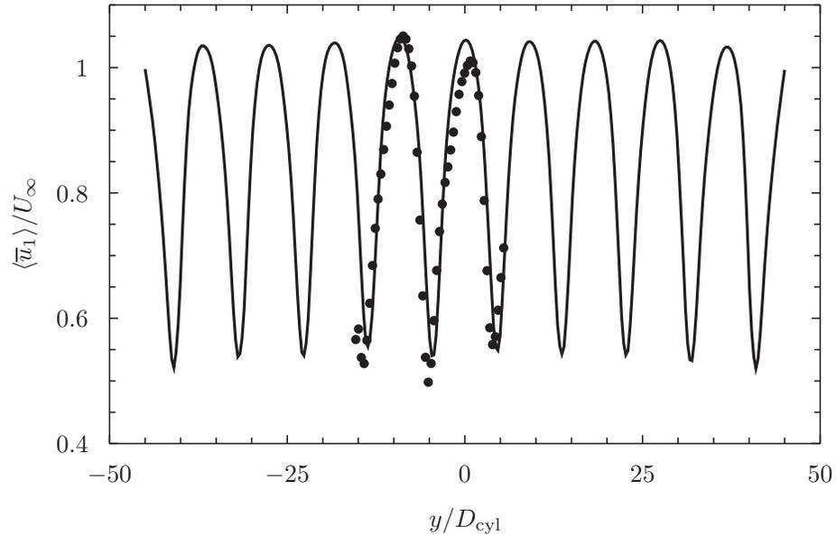
FIGURE 8. Mean velocity profiles as a function of the spanwise coordinate  $y/D$  for an array of stationary cylinders, taken at a height  $z/H = 0.43$  and taken at the same height,  $z/H = 0.43$ , and taken between the fifth and sixth cylinder in the array. The line is the result from the modeled computation and the symbols are from the experiment of Craig *et al.* (2013).
