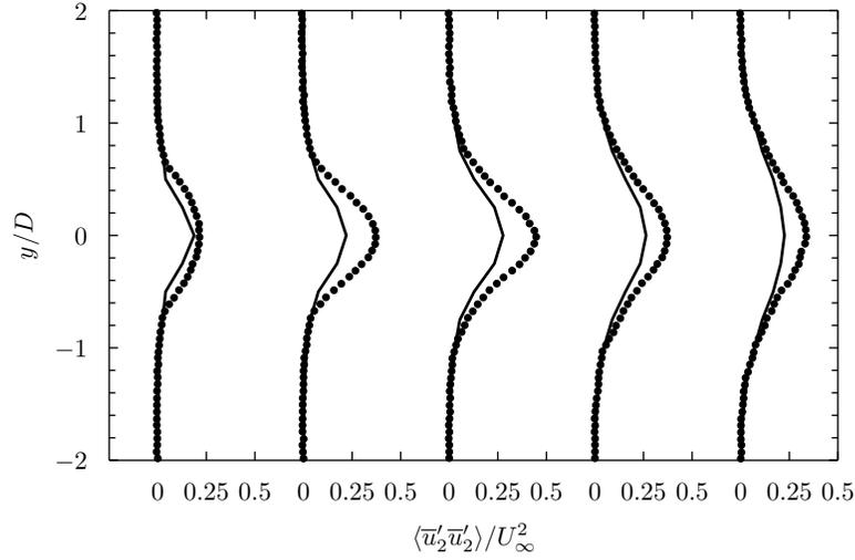
FIGURE 3. Mean vertical velocity fluctuation profiles,  $\langle \bar{u}'_1 \rangle$  as a function of vertical coordinate  $y/D$  at various locations  $x/D = 1.2, 1.5, 2.0, 2.5, 3.0$ , with  $x/D = 0$  corresponding to the cylinder center for a stationary cylinder. The lines are the results for the modeled computation, and the symbols are from the DNS of Mittal & Balachandar (1997).
