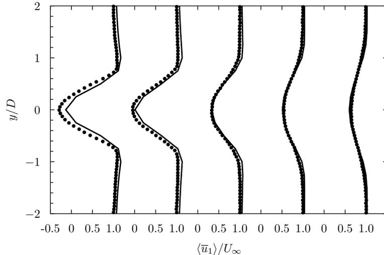
FIGURE 1. Mean streamwise velocity profiles,  $\langle \bar{u}_1 \rangle$  as a function of vertical coordinate  $y/D$  at various locations  $x/D = 1.2, 1.5, 2.0, 2.5, 3.0$  from left to right, with  $x/D = 0$  corresponding to the cylinder center for a stationary cylinder. The lines are the results for the modeled computation, and the symbols are from the DNS of Mittal & Balachandar (1997).
