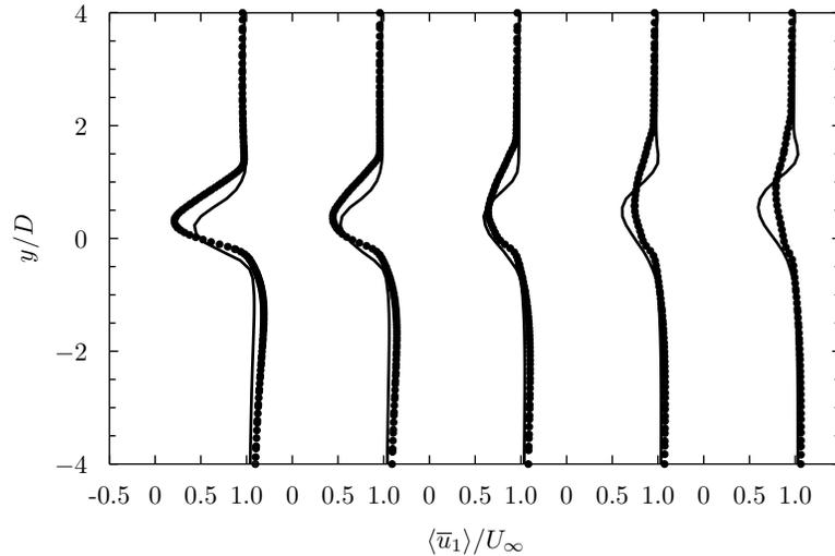
FIGURE 4. Mean streamwise velocity profiles,  $\langle \bar{u}_1 \rangle$  as a function of vertical coordinate  $y/D$  at various locations  $x/D = 1.2, 1.5, 2.0, 2.5, 3.0$ , with  $x/D = 0$  corresponding to the cylinder center for a cylinder with  $\hat{\Omega} = 1.5$ . The lines are the results for the modeled computation, and the symbols are from our DNS.
