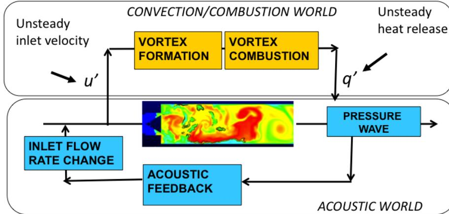
FIGURE 4. The paradigm used in TA codes. The instability loop is closed in two parts: a convective one containing also reaction and an acoustic one.
