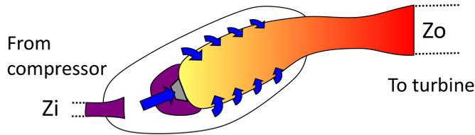
FIGURE 3. Acoustic impedances in a real gas turbine chamber. The unstable modes of the chamber cannot be computed without taking into account the acoustic effects of the compressor (left) and the turbine (right) which are usually quantified by their impedances  $Z_i$  and  $Z_o$ .
