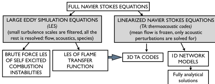
FIGURE 2. Methods to study combustion instabilities.
