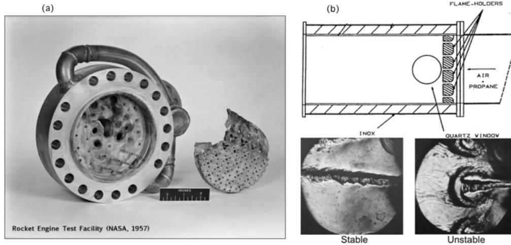
FIGURE 1. Combustion instabilities. (a): a rocket chamber destroyed by an unstable mode, (b): visualization of stable and unstable modes in a laboratory rig (Poinsot *et al.* 1987).
