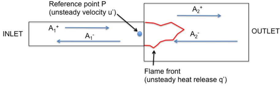
FIGURE 5. An illustration of wave propagation in a combustor. The  $A_1^-$  and  $A_2^+$  waves cannot influence the unsteady reaction for causality reasons.
