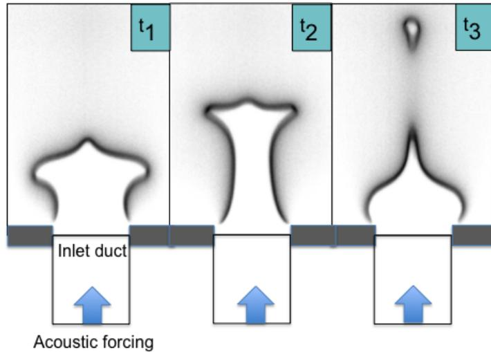
FIGURE 6. FTF measurement in a laminar configuration. Flame position (experimental result) during a forcing cycle at three instants (PhD thesis of Y. Dhue, IMFT).
