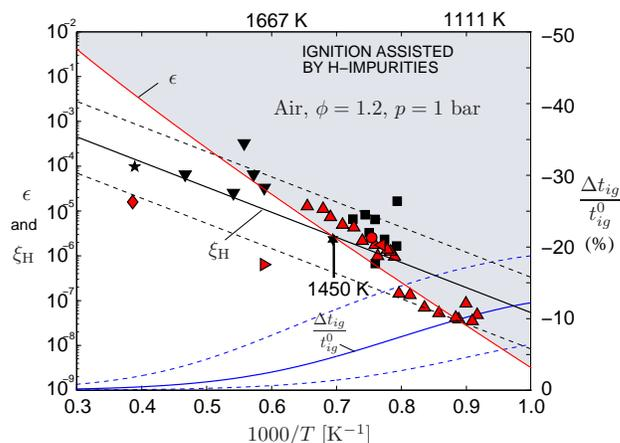
FIGURE 3. Effects of uncertainties in the residual impurities on the autoignition time variations (4.11) calculated from the solution to the reduced-order ignition problem (4.1)-(4.3) subject to (4.6). Solid and dashed lines indicate mean and mean  $\pm$  standard deviation respectively. The symbols denote the same experimental data points shown in Figure 2.
