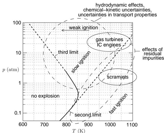
FIGURE 1. Explosion diagram for stoichiometric  $\text{H}_2/\text{O}_2$  mixtures (adapted from Lewis & von Elbe (1961)). The diagram includes typical operating conditions in propulsion systems, as well as some of the dominant effects that induce uncertainties in shock-tube measurements and computations of  $\text{H}_2/\text{O}_2$  ignition.
