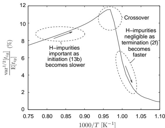
FIGURE 5. Dimensionless standard deviation induced by the uncertainties in H-impurities on the ignition time calculated using the Stanford mechanism Hong *et al.* (2011) after  $2 \cdot 10^5$  samples, for  $\text{H}_2/\text{air}$ ,  $\phi = 1.0$  and  $p = 2.5$  bar. The mean deviation  $E[t_{ig}] - t_{ig}^0$  follows a similar trend with decreasing temperature as the standard deviation shown here.
