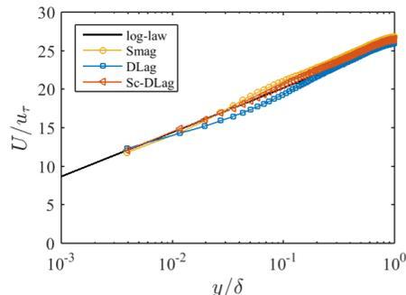
FIGURE 1. Mean velocity profile for WMLES. The sub-grid stress is modeled using the standard constant coefficient Smagorinsky model (Smag), the dynamic Lagrangian averaged model (DLag) and the scale-dependent version of the dynamic Lagrangian averaged model (Sc-DLag). The equilibrium wall model is used for near-wall closure. The grid size of the LES in this plot is  $128^3$ . The detailed LES setup is discussed in detail in Section 4.1.
