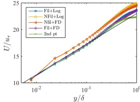
FIGURE 6. Mean velocity profile from various WMLES calculations. Fil is filtering at the first grid point, NFil is no filtering at the first grid point, Log is computing derivatives at the first grid point from the wall model, FD is computing derivatives at the first grid point using 2nd order finite difference (the same as in the bulk), 2nd pt is using the 2nd point for the wall model LES matching location.
