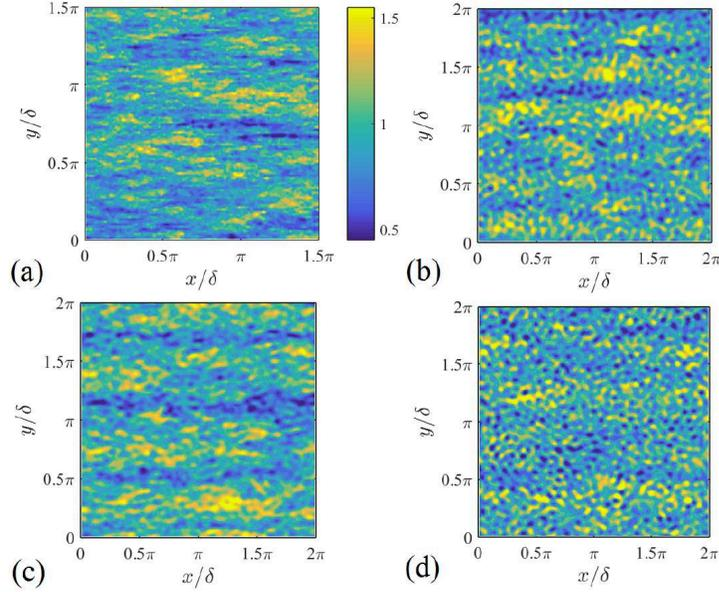
FIGURE 4. Contour plots of the normalized instantaneous streamwise wall shear stress,  $\tau_{w,x}/u_\tau^2$  from (a) the filtered DNS (b) the LES modeled by the equilibrium wall model (c) the integral wall model and (d) the non-equilibrium slip-wall model. All LES cases are run with a grid size of  $128^3$ .
