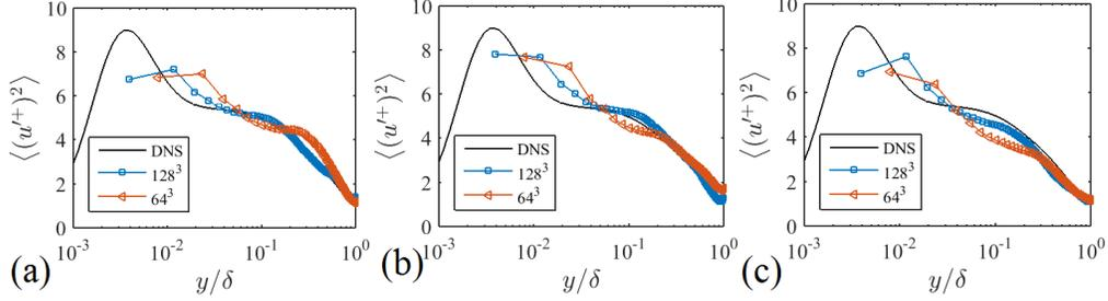
FIGURE 3. Variance of the streamwise velocity fluctuations plotted against the wall-normal distance for (a) the algebraic equilibrium wall model, (b) the integral wall model, (c) the equilibrium slip-wall model. DNS data are shown for comparison.
