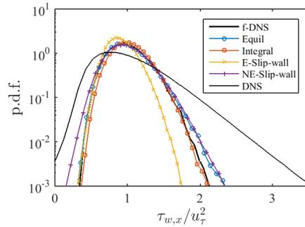
FIGURE 5. The streamwise wall stress PDF from WMLES, DNS and filtered DNS. f-DNS is filtered DNS. The other legends are the same as those in figure 2.
