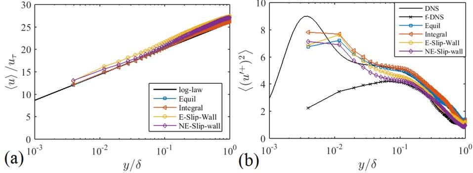
FIGURE 2. (a) Mean velocity profiles plotted against the wall-normal distance.  $\delta$  is the half-channel height. The log-law corresponds to  $U/u_\tau = 1/\kappa \log(yu_\tau/\nu) + B$ , with  $\kappa = 0.4$ ,  $B = 5$ . Equil is the algebraic equilibrium wall model, Integral is the integral wall model, E-Slip-Wall is the equilibrium slip-wall model, NE-Slip-Wall is the non-equilibrium slip-wall closure and f-DNS is the filtered DNS. (b) Same as (a) but for the streamwise variance.
