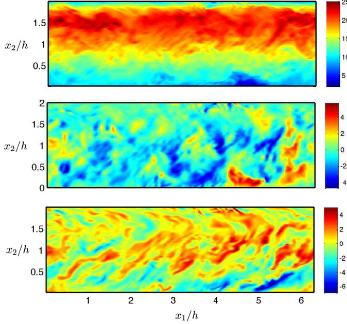
FIGURE 2. Instantaneous  $x_1$ - $x_2$  plane of the streamwise (top), wall-normal (center) and spanwise (bottom) velocities in a spanwise rotating channel flow with slip boundary conditions at the walls for  $Re_\tau = 395$  and  $Ro_\tau = 10$ . The colorbar shows velocity in wall units.
