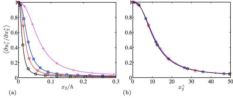
FIGURE 1. Mean viscous stress as a function of the wall-normal direction  $x_2$  in (a) outer units and (b) wall units for four different Reynolds numbers in a turbulent channel flow. Symbols are equal to  $\text{Re}_\tau$  as follows: +, 180; □, 395; ▽, 546; ○, 932. Data from del Álamo *et al.* (2004) and Lozano-Durán & Jiménez (2014).
