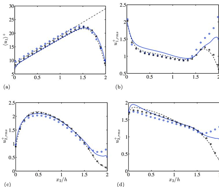
FIGURE 4. (a) Mean streamwise velocity profile. (b) Streamwise, (c) wall-normal and (d) spanwise rms velocity fluctuations. Lines are DNS at  $Re_\tau = 180$  (dashed) and 395 (solid). Symbols are LES at  $Re_\tau = 180$  ( $\square$ ) and 395 ( $\circ$ ). The dash-dotted line in (a) has the slope  $2\Omega$ .
