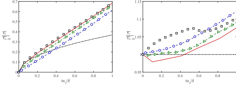
FIGURE 3. Time history of the mean spanwise ( $\overline{\tau_3}$ , left) and streamwise ( $\overline{\tau_1}$ , right) wall shear-stress vector components from WMLESs and the DNS. Both terms have been normalized by the initial 2D wall shear-stress value ( $\overline{\tau_{w,2D}}$ ). Red solid line, DNS; square symbols, WMLES (NEQWM); triangle symbols, WMLES (IWM); circle symbols, WMLES (EWQM); black dash-dotted line, laminar solution.
