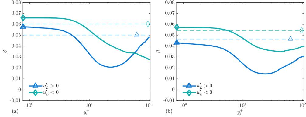
FIGURE 4.  $\beta_{\leq}$  [measured according to Eqs. (3.2)-(3.3)] as functions of  $y_i^+$  for channel flow at  $Re_\tau = 2000$  (solid lines). Dashed lines represent the predictions using Eq. (3.4). (a) for  $y_o^+ = 215$  and (b) for 400.
