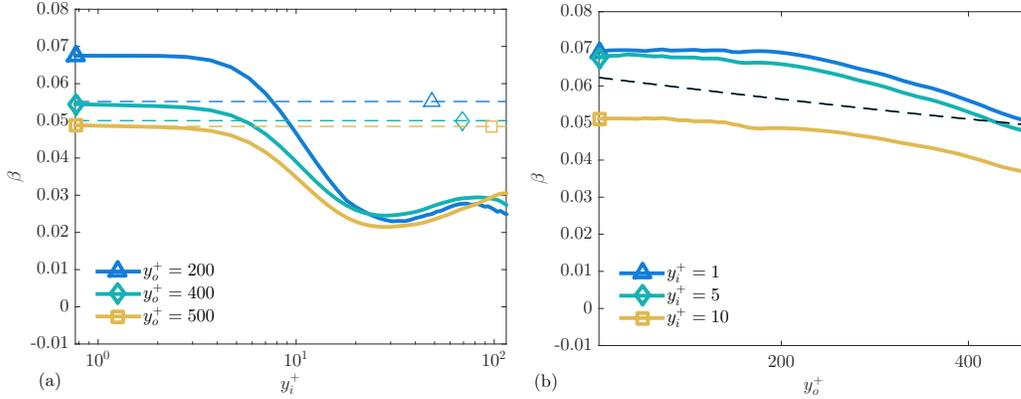
FIGURE 1. (a) The amplitude modulation coefficient  $\beta$  as functions of  $y_i^+$  for three outer locations,  $y_o^+ = 200, 400$ , and  $500$  ( $y_o/\delta = 0.1, 0.2$ , and  $0.25$ ). The  $Re_\tau = 2000$  channel flow direct numerical simulation (Hoyas & Jiménez 2006) is used for the measurements.  $\beta$ , as suggested by Eq. (2.8), is indicated using dashed lines. (b)  $\beta$  as functions of  $y_o^+$  for  $y_i^+ = 1, 5$ , and  $10$ .
